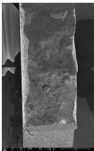
Brut-R1-ST4 A = 3.70 \% / R_m = 952 \text{ MPa} Hv_{2kgs} = 370.92 \pm 12.61
