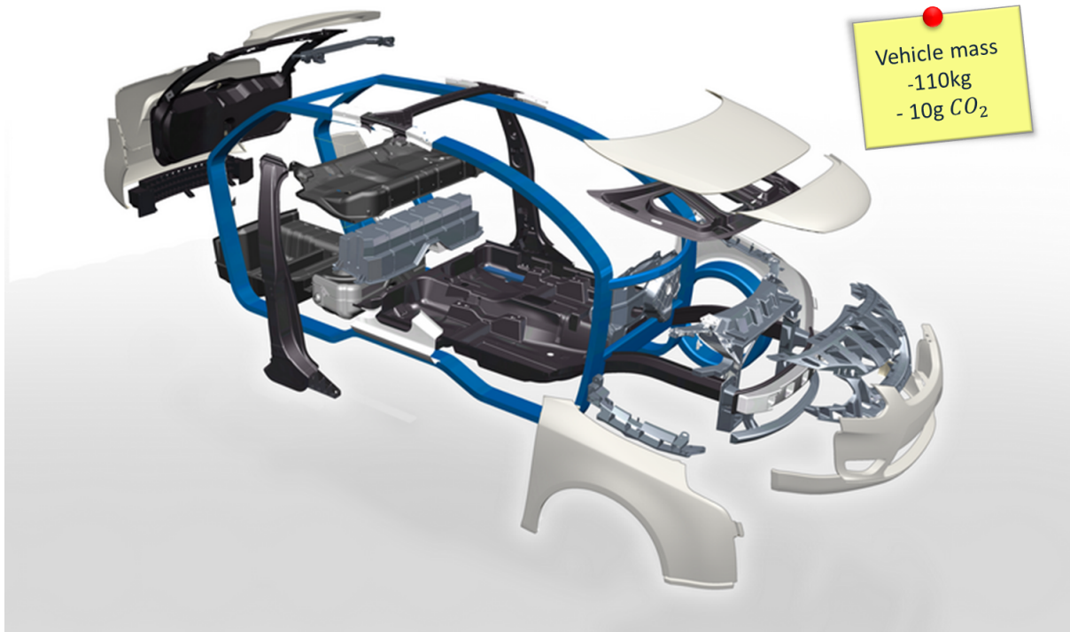
Figure 3: View of potential parts to be replaced by fiber reinforced composites in order to gain up to 110Kg of weight saving. In white the parts conceding the exterior bodywork, the gray stands for structural parts and the black for semi-structural parts. (Image courtesy of Plastic Omnium)
