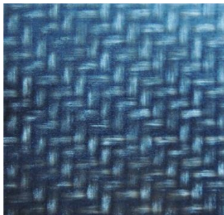
Figure 2-1 Bond Laminates TEPEX dynalite 102-RG600(x)/45% Roving Glass – PA 6.
