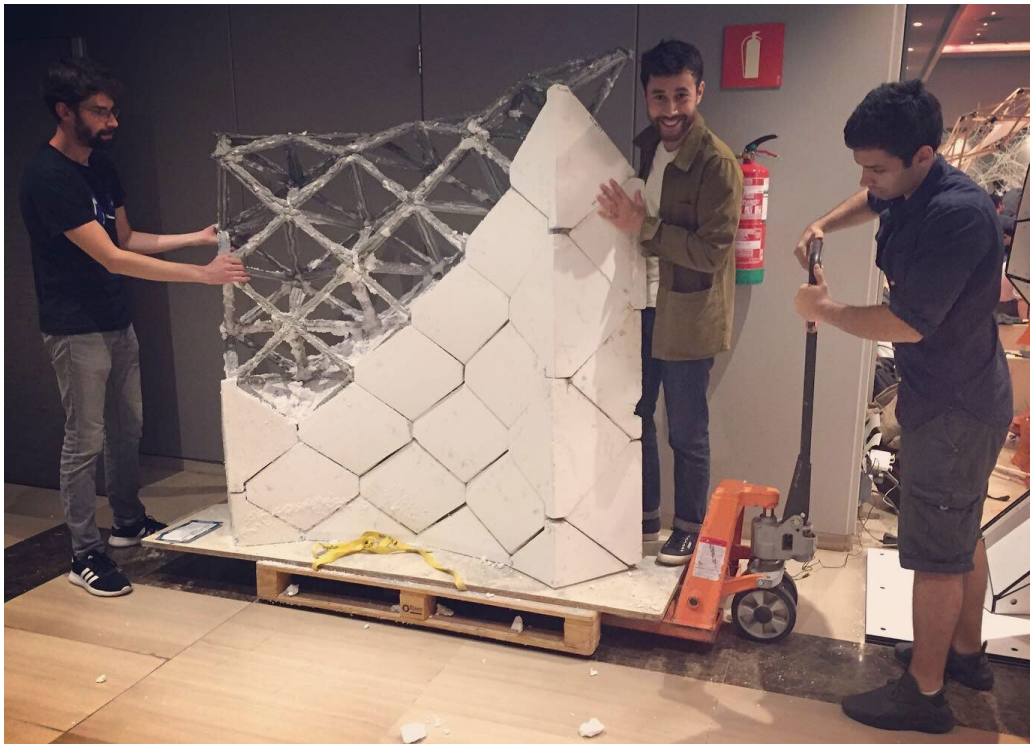
Figure 3.6. The curved version of the space-truss wall with continuous fiber reinforcement presented on the IASS 2019 symposium
