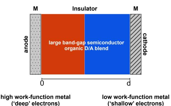
Figure 1.6 – Schematic depiction of a MIM junction that best captures the general working principle of an organic solar cell. The left electrode is the anode while the right electrode is the cathode.
