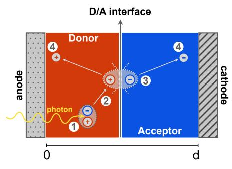
Figure 1.1 – Illustration depicting all the 4 steps in which the photovoltaic process may be divided. (1) photon absorption and exciton generation, (2) exciton diffusion and encounter with the interface (3) exciton dissociation (4) charge collection at the electrodes.
