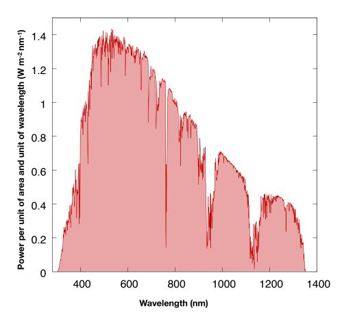
Figure 1.4 – Sun spectrum after being filtered by an air mass equivalent to the atmosphere crossed by rays at  $48.2^{\circ}$  of zenith angle. Conventionally this condition is referred to as "solar spectrum AM 1.5".
