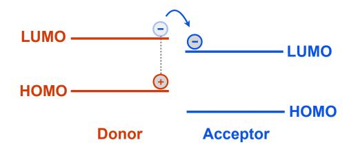
Figure 1.2 – Matching of the energy levels at the donor acceptor interface that ensure the dissociation of the exciton into free charges. This is valid for both planar and bulk heterojunction. Any neighbouring pair of a donor and an acceptor may realise the exchange according to this scheme.
