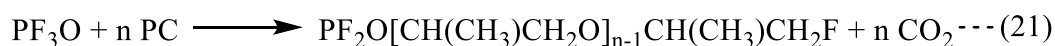
Scheme. 1 Reduction reactions on Si thin film electrode with different electrolytes (1 M LiPF 6 /EC-DMC, 1 M LiPF 6 /DMC and 1 M LiPF 6 /PC).
