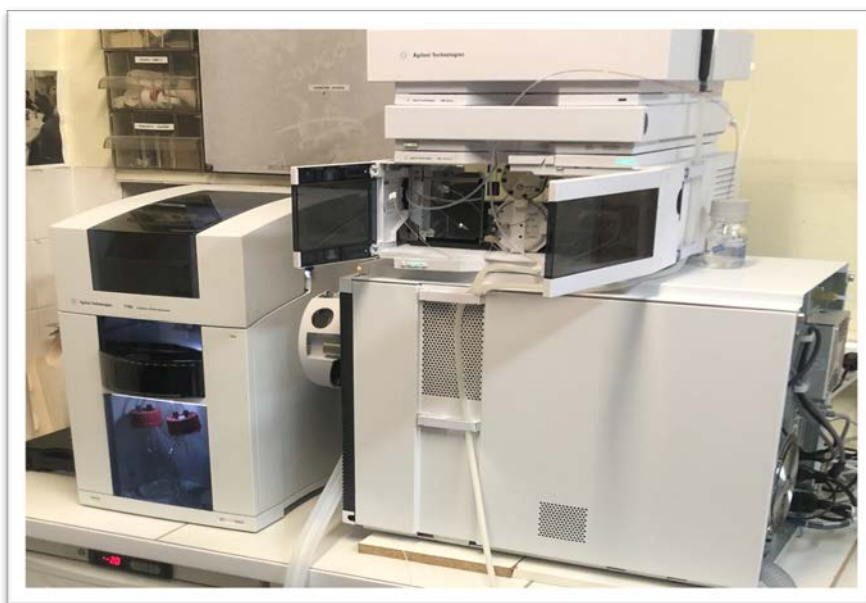
Figure 2.1: CE-ESI MS instrumentation used for the separation of the QDs synthesized in this work.
