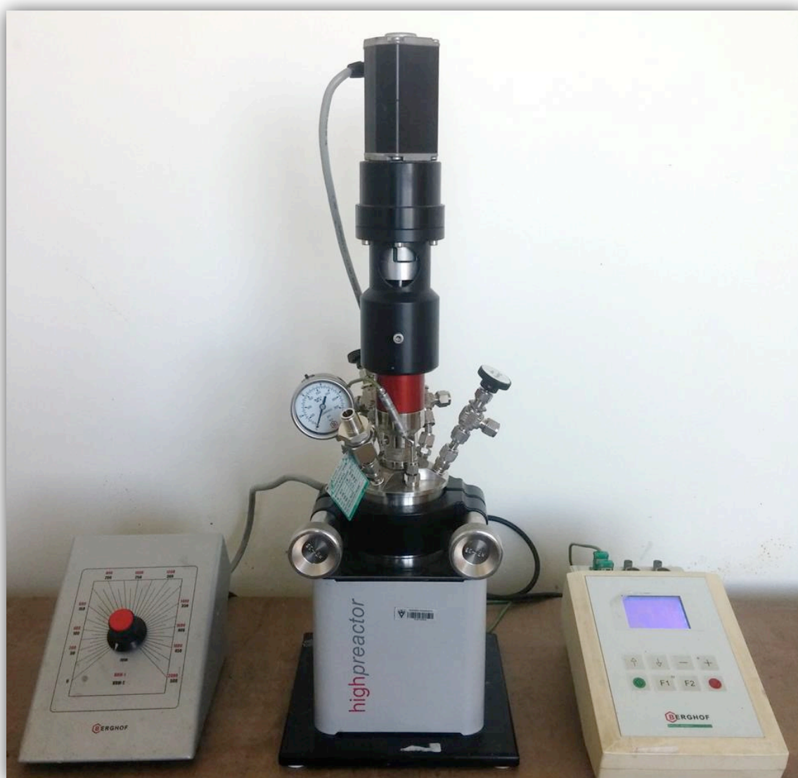
Fig. 2.2: Berghof high pressure reactor employed for the hydrothermal synthesis of the QDs used in this work.
