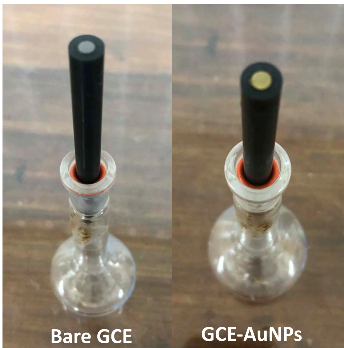
Figure 4.5: Images of a bare GCE and the GCE after cycling in 1 mM \text{HAuCl}_4 in 0.1 M \text{NaNO}_3 .
