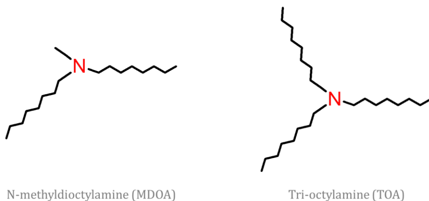
Figure 1.7 Comparison between the chemical structure of N-methyldioctylamine with tri-octylamine
