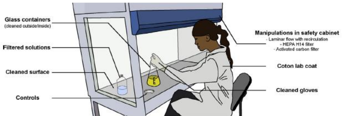
Fig. 2. Representation of basic precautions to avoid sample contamination in the context of MP load analysis.
