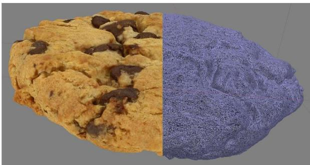
**Fig. 2.** Realism of a virtual cookie (“Co”) after Agisoft Photoscan® 3D reconstruction.
