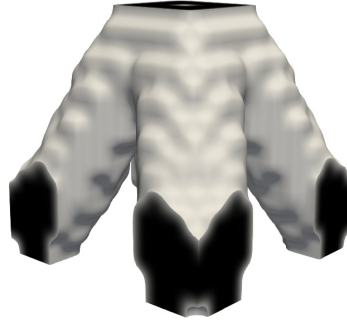
(a) B-spline with p_1 = p_2 = p_3 = 2 and n_1 = n_2 = n_3 = 4 , N_{\text{iter}} = 500 , d_{\text{min-meas}} = 14.7 mm
