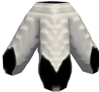
(b) NURBS with p_1 = p_2 = p_3 = 2 and n_1 = n_2 = n_3 = 4 , N_{\text{iter}} = 500 , d_{\text{min-meas}} = 12.6 mm
