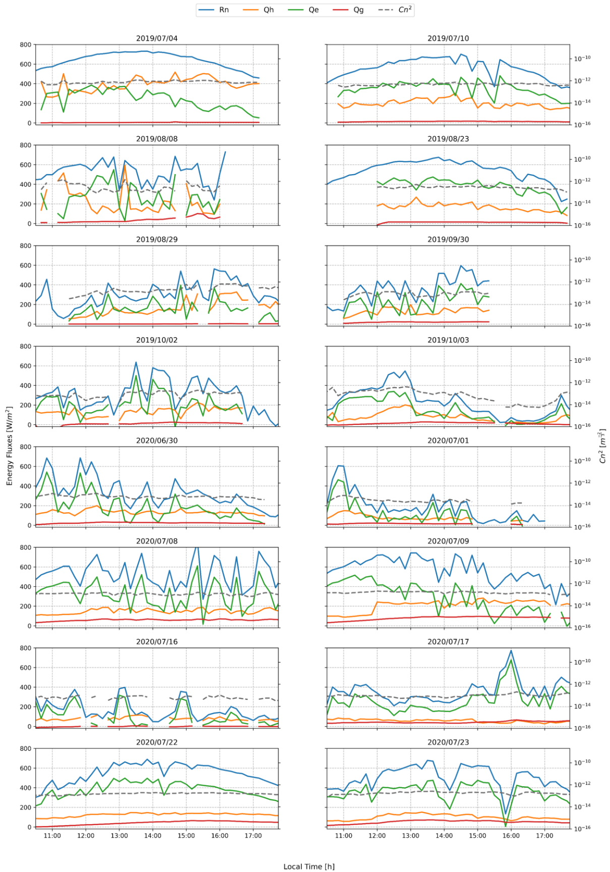
Figure 2.15. Surface Energy Balance (SEB) and C_n^2 from LAS.
