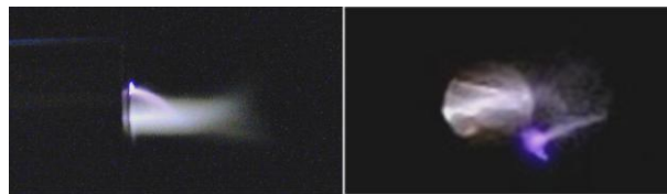
Figure 8. Fast camera photograph of the plasma arc at the tip of the nozzle. Left: side view. Right: Front view. I = 0.25 A. Q_{\text{air}} = 0.32 \text{gs}^{-1} .
