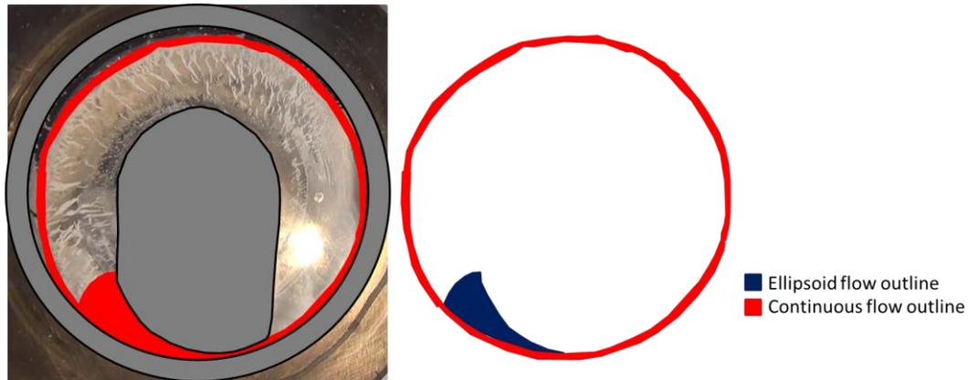
**Figure 4.8** – Ellipsoid and continuous flow outline of SBR A at 5 rpm and 100°C with the transparent Monocuve mixer.
