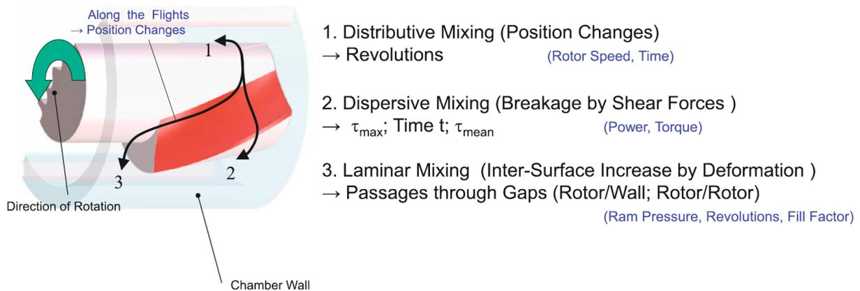
**Figure 1.7** – Flow paths within the internal mixing due to rotor wing design providing distributive, dispersive and laminar mixing [Limper, 2012].
