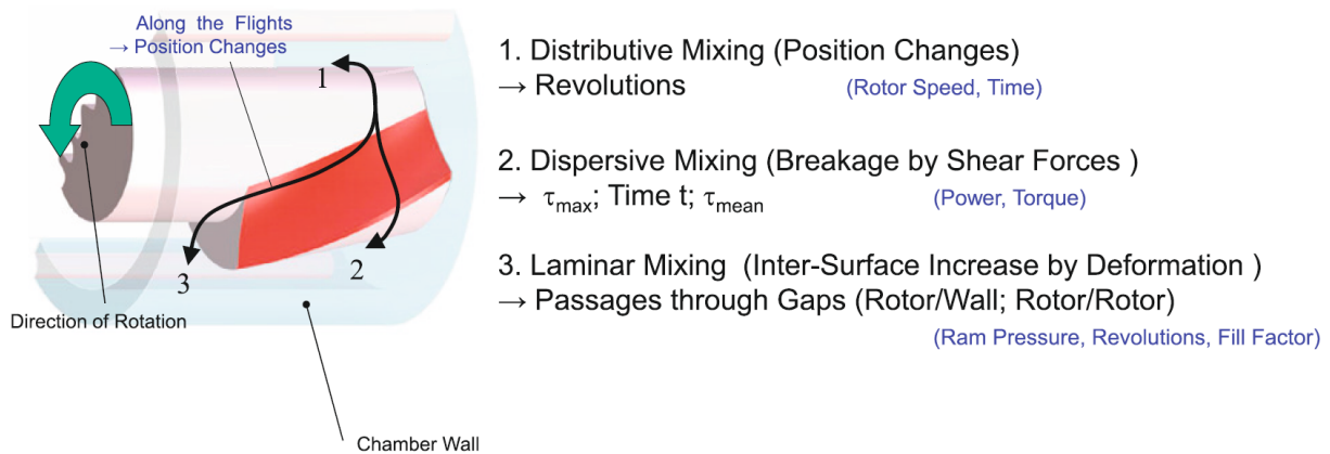
Figure 1.7 – Flow paths within the internal mixing due to rotor wing design providing distributive, dispersive and laminar mixing [Limper, 2012].
