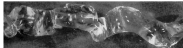
Figure 1.15 – Different types of extrusion defects [Agassant et al. , 2014].
