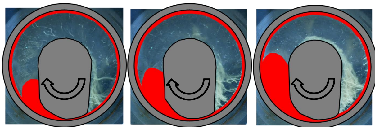
Figure 4.10 – Flow observations of SBR B in the Monocuve mixer at 20 rpm, 100°C and at 20% (Left), 25% (Middle) and 35% (Right) volume fill factors.
