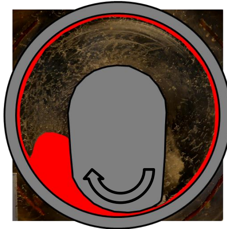
Figure 4.14 – Flow observations of the silicone fluid in the Monocuve mixer at 25% volume fill factor, 2 rpm and at ambient temperature.
