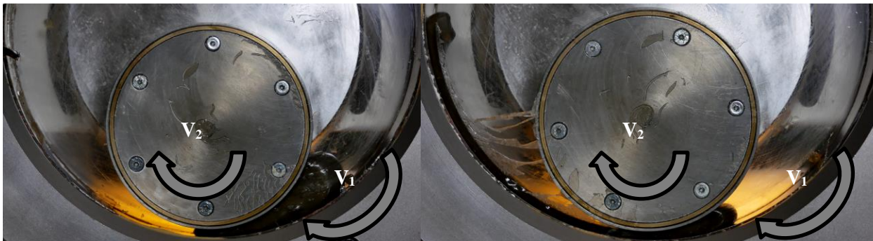
Figure 4.22 – Flow observations in co-rotation condition at small fill factors a) before passing through the thin flow gap and b) after passing through the thin flow gap.
