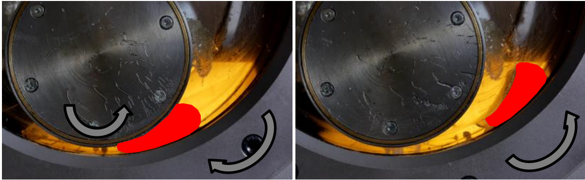
Figure 4.29 – Dewetting of the inner cylinder surface indicating unilateral contact of the fluid with the cylinder surfaces.
