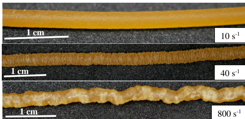
Figure 3.41 – Flow extrudates of SBR B at 100°C for a capillary die of L/D = 8 and D = 2 mm.
