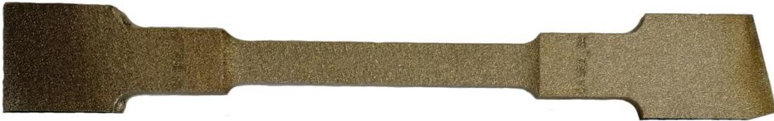
Fig. 2-11 Typical sample, as received from Safran. The specimen is in its rough state, after LPBF processing, and separation by Electrical discharge machining (EDM) from the build plateau.
