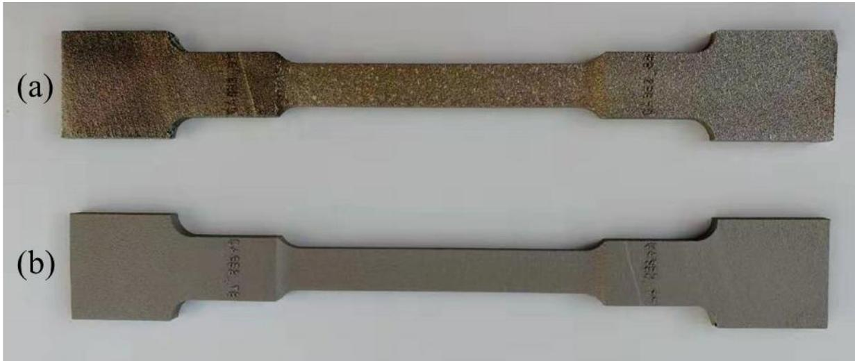
Fig. 2-13 Surface state of sample. (a): as received, and (b): after sandblasting
