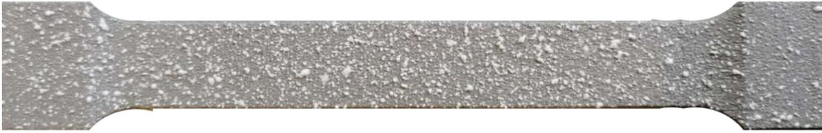
Fig. 2- 15 Sample with speckle prepared by brush spattering
