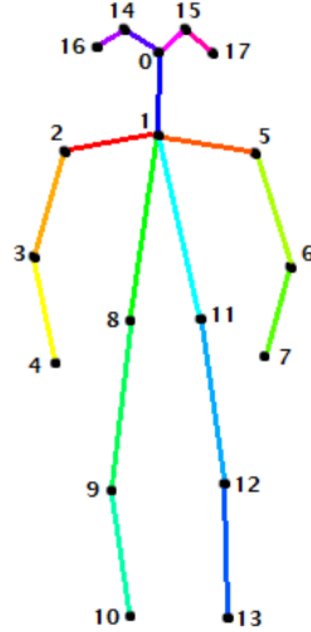
Figure 2.19: Data structure of the skeleton representation obtained with the OpenPose library [Cao et al., 2017]
