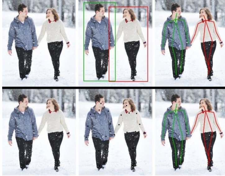
Figure 2.10: Top down : consists of adding a person detector in order to identify all the articulations (keypoints) of each person and then estimate the pose according to them. Bottom up : consists of detecting all the keypoints in the image ( i.e the limbs of each person), then associating these keypoints with their respective owners. Picture Credit [BeyondMinds, 2020]
