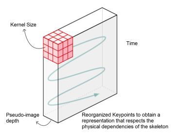
Figure 2.20: Kernel of a 2D convolution sliding over the pseudo-image
