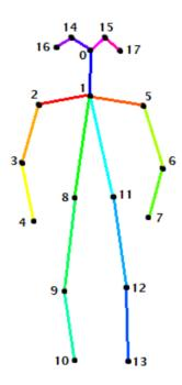
Figure 2.19: Data structure of the skeleton representation obtained with the OpenPose library [Cao et al., 2017]
