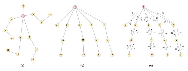
Figure 2.21: (a) Joints of the skeleton of a human body with the initial data structure (14 keypoints). The visiting order of the nodes is incremental:0-1-2-3-...-13. (b) The skeleton is transformed into a tree structure. (c) The tree can be unfolded into a chain whose order of visit of the nodes maintains the physical relationship of the joints: 1-0-1-8-10-12-10-8-1-9-11-13-11-9-1-2-4-6-4-2-1-3-5-7-5-3 (26 keypoints).
