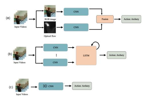
Figure 2.6: Illustration of RGB-based deep learning methods for action recognition: (a): two-stream 2D CNN-based methods, (b) RNN-based methods, (c) 3D CNN-based methods. Image adapted from [Sun et al., 2020].
