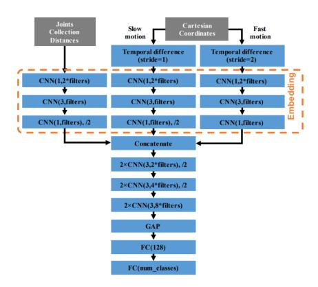
Figure 2.22: The network architecture of DD-Net [Yang et al., 2019]. "2×CNN(3, 2\*filters), /2" denotes two 1D ConvNet layers (kernel size = 3, channels = 2\*filters) and Maxpooling (strides = 2). Other convolutive layers are defined in the same format. GAP denotes Global Average Pooling. FC denotes Fully Connected Layers. We can change the model size by modifying the "filters" parameter.
