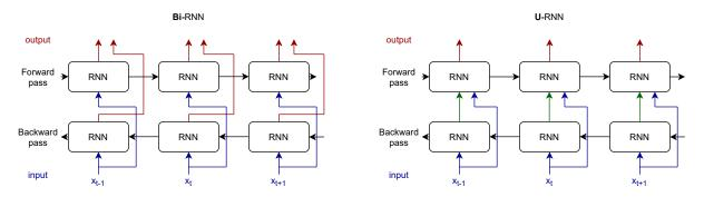
Figure 3.4: Comparison between Bi-RNN and U-RNN architectures (blue: inputs - red: outputs - black: hidden states - green: intermediate output). U-RNN can use the information from the future during the forward pass, whereas the Bi-RNN only concatenates two naive readings in both directions.
