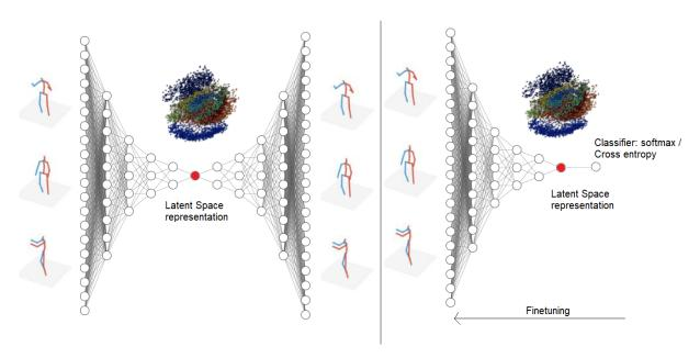
Figure 2.14: Pipeline of the approach: (1) we train an auto-encoder to reconstruct a sequence representing an action according to the evolution over time of the keypoints. We also add a constraint specific to the separability of classes in the latent space. (2) We then extract the weights of the encoder part up to the bottleneck represented in red and add a classifier, which transforms the encoder part into a pre-trained network on the data for action classification.
