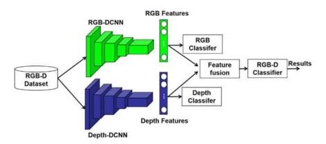
Figure 2.7: An Architecture of decision level fusion of RGB stream and Depth modalities. Picture credit [Gao et al., 2019]
