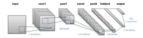
Figure 2.23: The architecture of the LeNet network [LeCun et al., 1998], with the basic components of a convolutional network: convolutions, pooling, fully connected layer and a softmax classifier.
