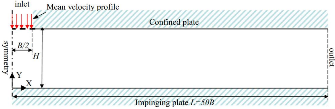
Figure 2.4: Setup of the jet impingement case
