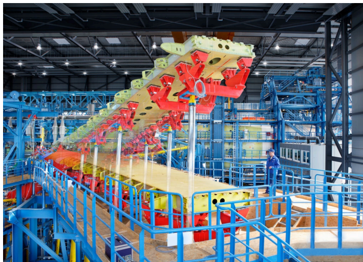
FIGURE 1.2 – Example of a fatigue test conducted on the wing of a plane in which the real loading conditions are reproduced to assess the mechanical part behavior under fatigue - case of the wing of an Airbus TM A380.
