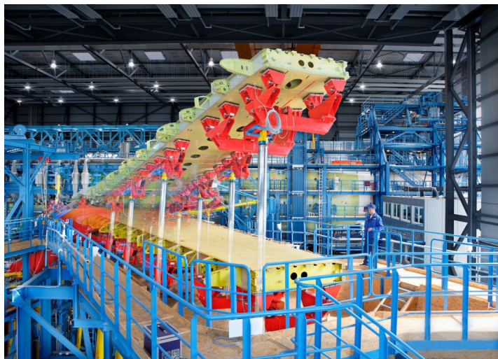
FIGURE 1.2 – Example of a fatigue test conducted on the wing of a plane in which the real loading conditions are reproduced to assess the mechanical part behavior under fatigue - case of the wing of an Airbus TM A380.
