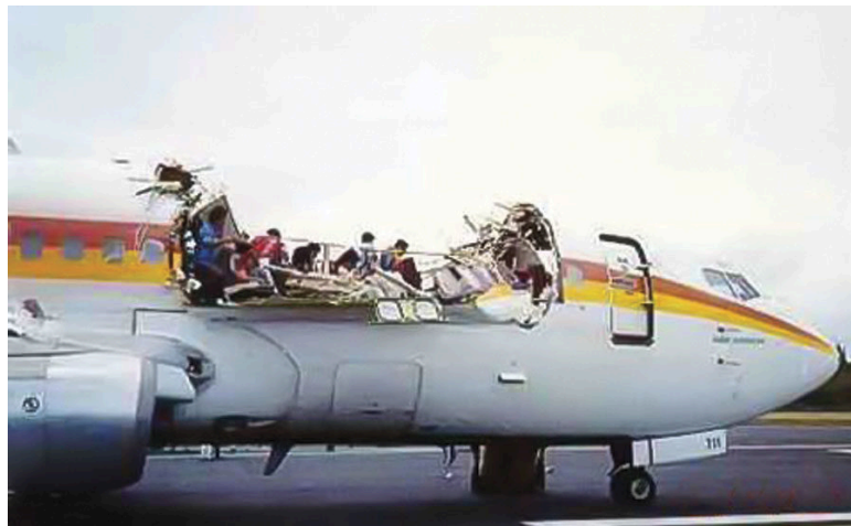
FIGURE 1.1 – Image of a broken plane fuselage (owing to a fatigue crack) [Jacek and Gieras, 2013].
