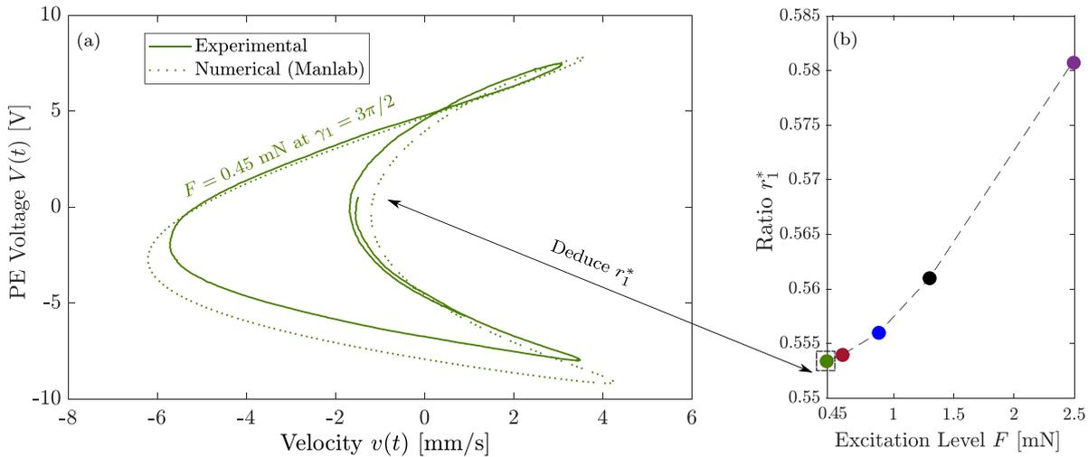
**Figure 14.** (a) Example of Lissajous plot for  $F = 0.45$  mN estimated numerically (with Manlab) and experimentally. (b) Deduced value of  $r_1^*$  for different excitation levels. The curves are estimated for  $\beta = 0.035$ ,  $\xi_e = 0.002$ , and  $\xi_1 = 0.005$ .
