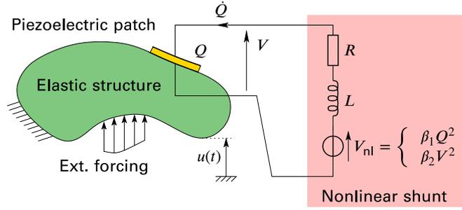
Fig. 1. Nonlinear shunt circuit.
