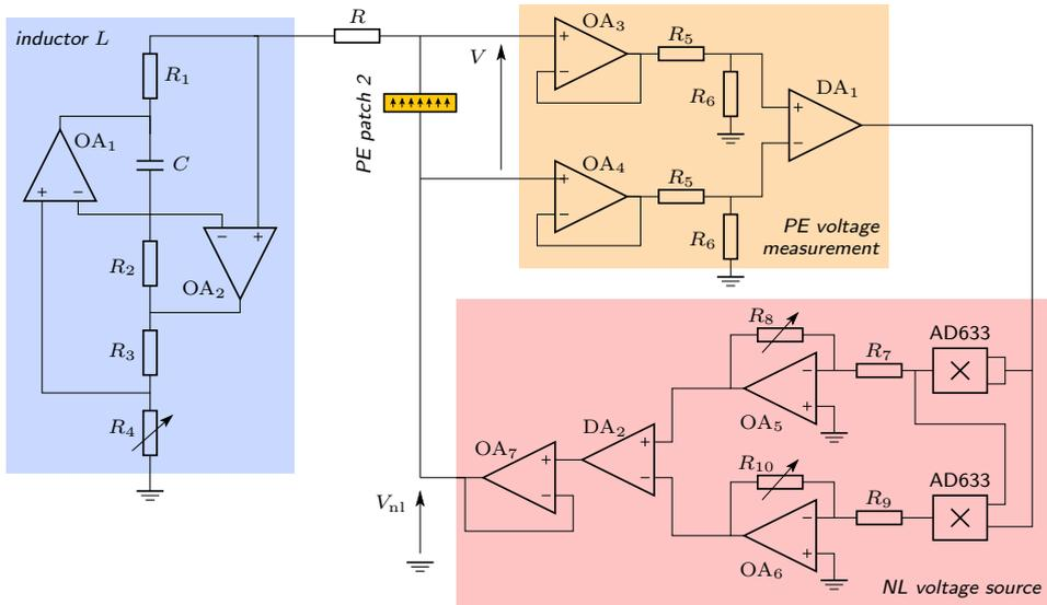
Figure 8: Nonlinear shunt circuit design.
