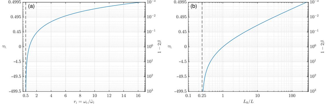
Fig. 8: Optimal value  $\beta^{\text{OP}}$  of  $\beta$  to tune the RL-shunt as a function of (a)  $r_i = \omega_e/\hat{\omega}_i$  and (b) as a function of the reduction ratio of the shunt inductance with respect to its optimal value for a linear RL-shunt  $L_0/L$ .
