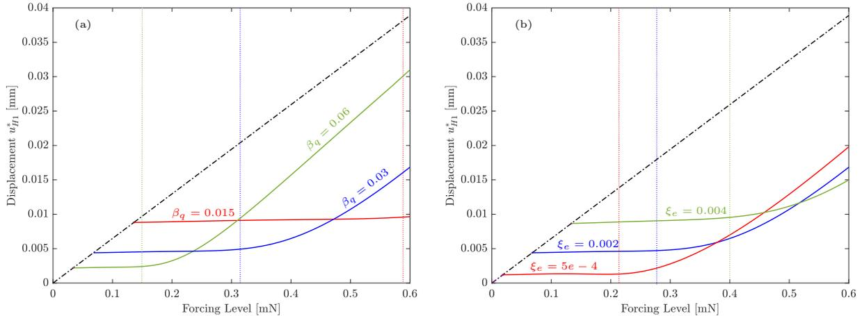
Figure 6: Displacement at the resonance frequency  $u_{H1}^*$  as function of the excitation level by considering the cubic component with  $\beta_c$  verifies Eq. (24) and  $r_1 = 0.5055$ . (a) for different values of  $\beta_q$  and (b) for different values of  $\xi_e$ . The modal parameters used are gathered in Table. 1. The dotted lines denote the maximum excitation level where the saturation is valid. The black dashed-dotted line denotes the linear response.
