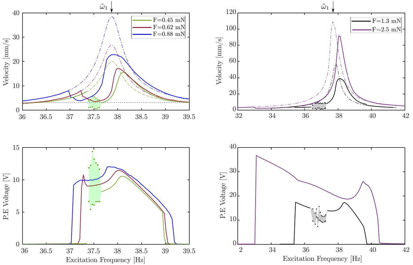
**Figure 13.** Experimental results of  $v_{H1}$  (first row) and  $V_{H1/2}$  (second row) for several excitation levels  $F$  with unit of mN. Only the data for sweeping down the excitation frequency are shown in solid lines. The measurements are done for  $\beta = 0.035$ ,  $\xi_e = 0.002$ ,  $\xi_1 = 0.005$ , and  $r_1 = 0.537$ . The shaded regions depict the detected quasi-periodic regime.
