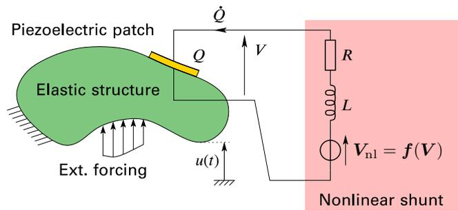
Figure 1.10: Nonlinear shunt circuit schematic with a nonlinear voltage source component  $V_{nl}$ .
