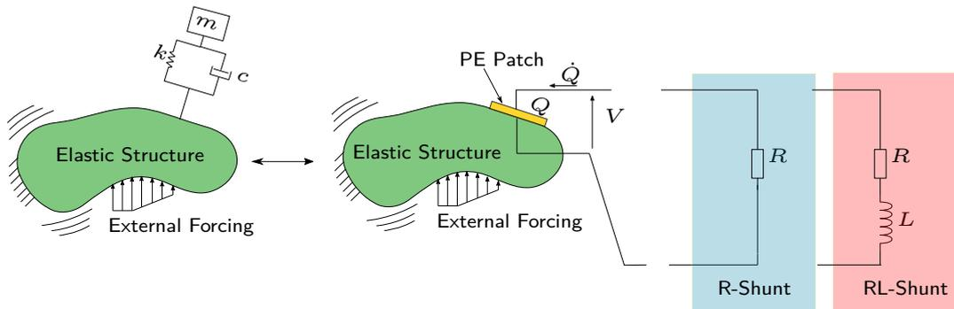
Figure 1.9: R-shunt and RL-shunt schematics. PE patch refers to a piezoelectric patch.  $Q$ ,  $\dot{Q}$ , and  $V$  are the charge in the piezoelectric electrode, the time derivative of the charge (i.e., the current), and the voltage across the PE patch.
