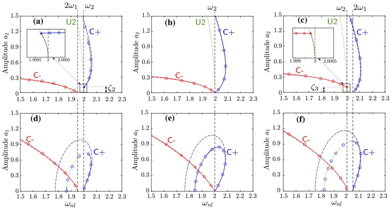
**Fig. 4** Backbone curves of the system with quadratic and cubic terms considered:  $g_{12}^1 = g_{11}^2 = 1$ ,  $g_{11}^1 = g_{22}^1 = g_{12}^2 = g_{22}^2 = 0.5$ , and  $h_{ijk}^p = 0.1$  for  $i, j, k$ , and  $p = 1, 2$ . Three different detunings are considered:  $\sigma = -0.05$  (first column),  $\sigma = 0$  (second column), and  $\sigma = 0.05$  (third column). Comparison between the second-order MSM result (dash-dotted) and the reference numerical solution directly
