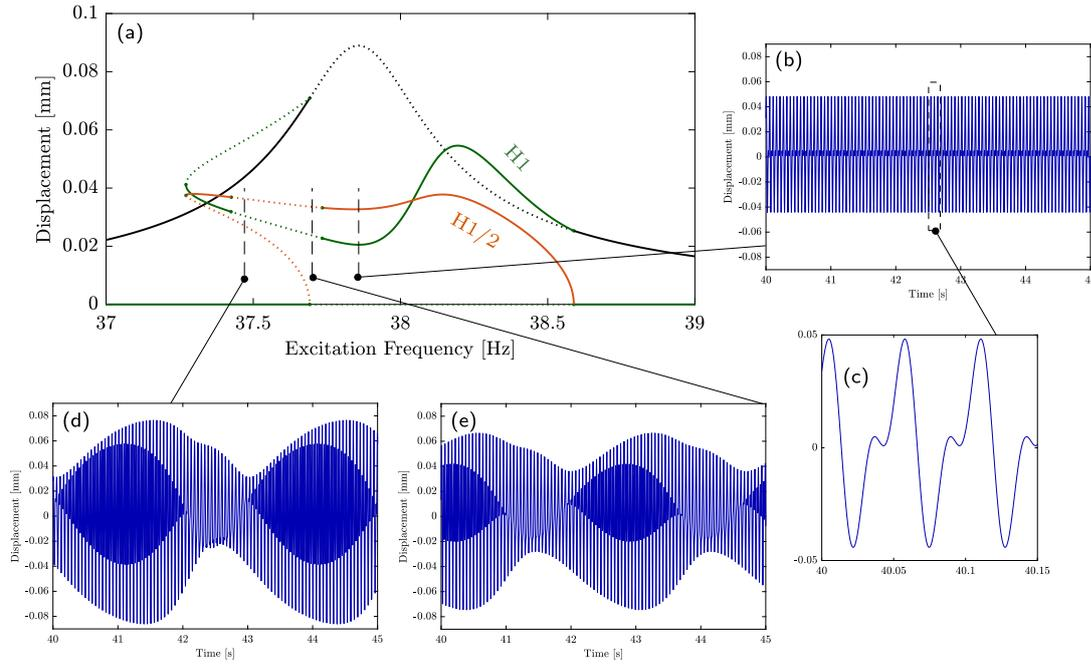
**Fig. 17.** (a) Resonant response around the first resonance of the beam with both the leading harmonics H1 and the subharmonic H1/2 of the beam's tip displacement (same case as Fig. 15 for  $\beta_2 = 0.015 \text{ V}^{-1}$ ); (b, c): periodic response at the antiresonance point; (d, e): examples of quasi-periodic responses, obtained by time integration. The parameters are those of Table 2, with  $F = 0.53 \text{ mN}$  and  $\xi_e = 0.0053$ .
