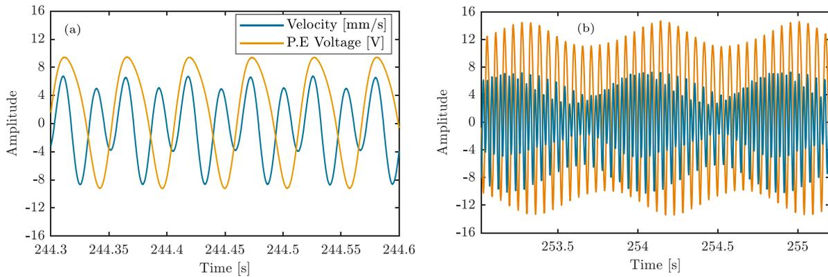
**Figure 11.** Experimental time signals of  $v(t)$  and  $V(t)$  for two frequency points in figure 10: (left) the periodic response at  $\Omega = 37.75$  Hz and (right) the QP regime at  $\Omega = 37.5$  Hz.
