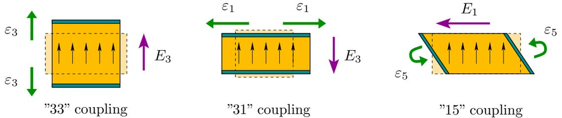
Figure 1.8: Piezoelectric coupling modes. Retrieved from [171].
