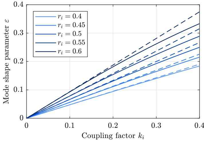
Fig. 13. Mode shape parameter  $\varepsilon$  as a function of the electromechanical coupling factor  $k_i$  for different values of the frequency ratio  $r_i$ , as specified. ‘—’: exact value from Eq. (14); ‘- -’: linear approximation, Eq. (46).
