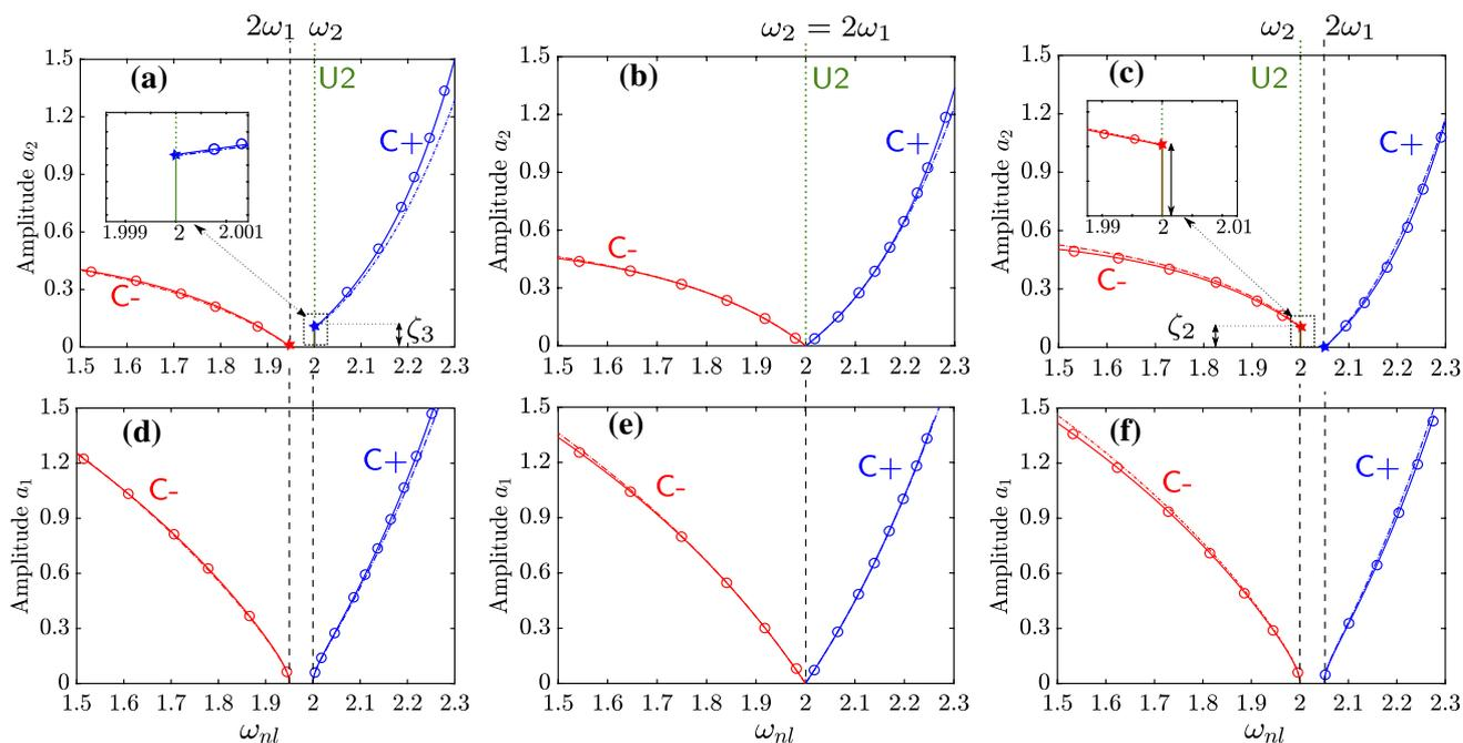
**Fig. 3** Backbone curves of the system in the specific case where only the quadratic resonant terms are considered such that  $g_{12}^1 = g_{11}^2 = 1$ , while the other nonlinear coefficients are zero. Three different detunings are analyzed:  $\sigma = -0.05$  (first column),  $\sigma = 0$  (second column), and  $\sigma = 0.05$  (third column). Comparison between the second-order MSM result (dash-
