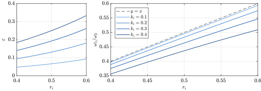
**Fig. 2.** (left) Mode shape parameter  $\varepsilon$  (from Eq. (14)) and (right) electromechanical natural frequency ratio  $\omega_1/\omega_2$  (from Eqs. (12)) as a function of the frequency ratio  $r_i$ , for various values of the EMMCF  $k_i$ , as specified.
