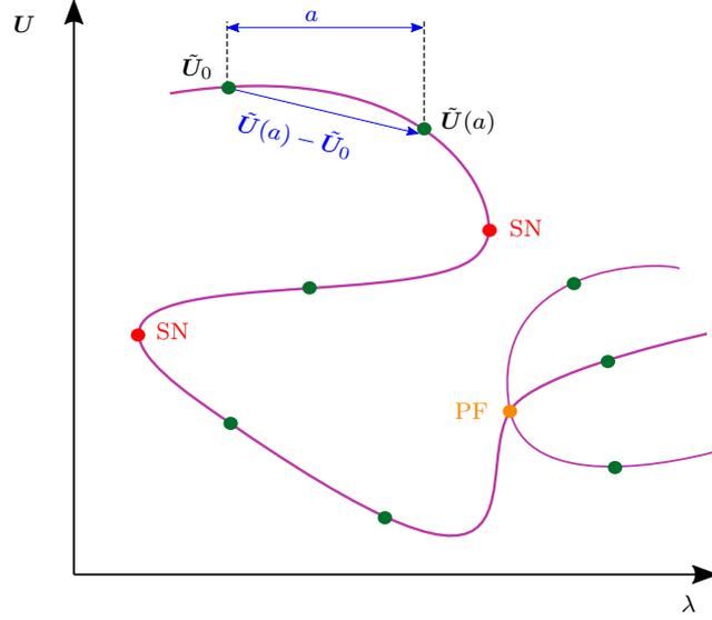
Figure 1.14: Bifurcation diagram of  $\mathbf{U}$  with respect to  $\lambda$ . The green dots denote the computations steps boundary according to  $a$ . The red and orange dots denote respectively the saddle-node bifurcations (SN) and Pitchfork bifurcations (PF).
