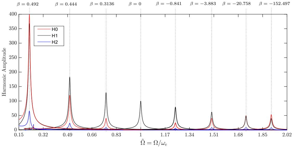
Fig. 3: Harmonics H0, H1 and H2 of the periodic solutions of Eq. (8) in the vicinity of the primary resonance, as a function of  $\tilde{\Omega} = \Omega/\omega_e$  for  $\xi_e = 0.005$ . The harmonics' amplitude is normalized with respect to the excitation level. The vertical dotted black lines show the value  $\bar{\omega}_e(\beta)$ .
