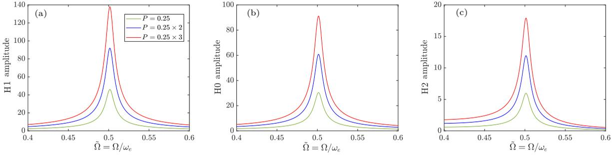
Fig. 4: Harmonics H1 (a), H0 (b) and H2 (c) of the periodic solutions of Eq. (8) in the vicinity of the primary resonance, as a function of  $\tilde{\Omega} = \Omega/\omega_e$  for  $\xi_e = 0.005$  and different excitation levels  $P$ . The numerical values used in the simulations are  $\xi_e = 0.005$  and  $\beta = 0.444$ .
