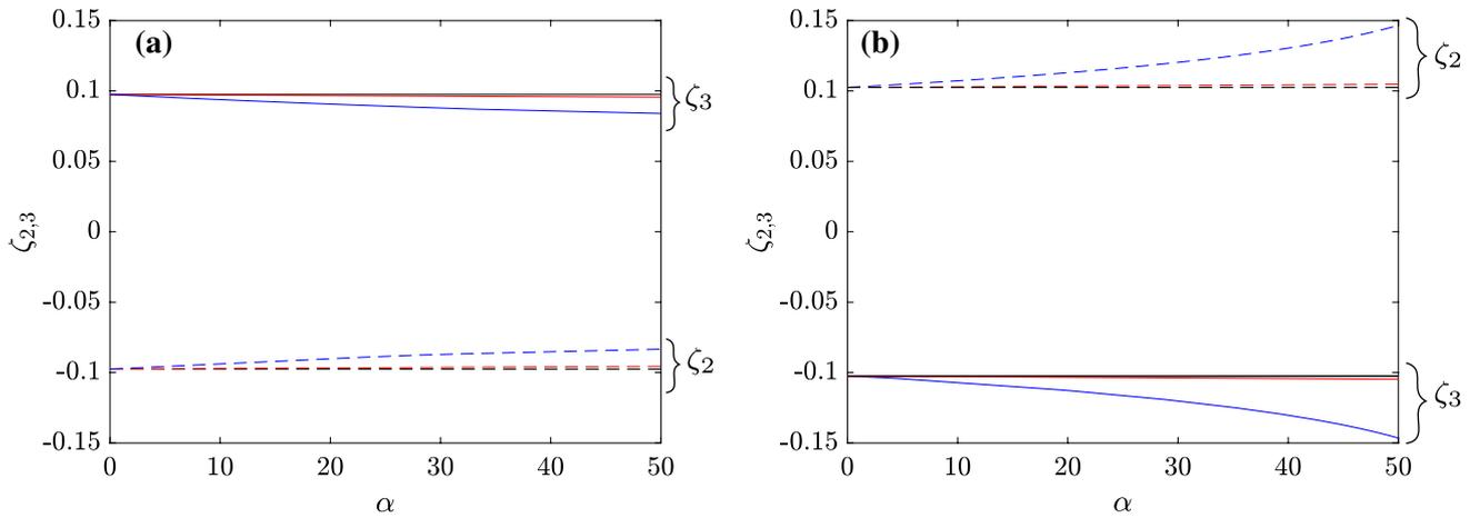
**Fig. 2** Behaviour of the roots  $\zeta_{2,3}$  as function of the cubic  $\alpha$  coefficient taken with equal values for simplicity ( $\alpha = \alpha_k \forall k$ ) and with  $\beta_1 = \beta_2 = 1$ . Solid lines refers to the C+ mode with  $p = 1$ , while dashed lines refers to the C- mode with  $p = -1$ . The red and blue lines denote respectively the case with  $\varepsilon = 0.001$
