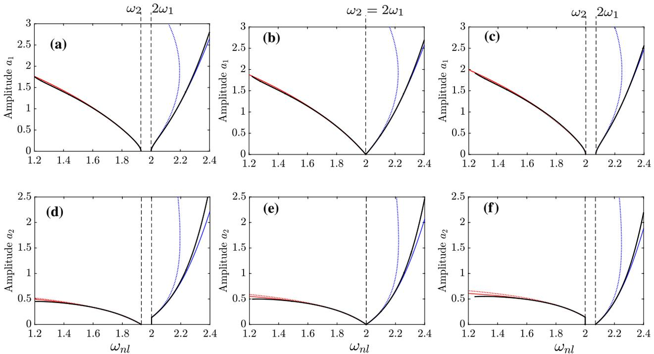
**Fig. 11** Comparison between the analytical results of the two approaches presented in (18a, b) and (87a, b) with the numerical results computed with Manlab. Only the quadratic resonant terms are considered such that  $g_{12}^1 = g_{11}^2 = 1$  with the other nonlinear coefficients are set to zero. The backbones are plotted in the planes  $(a_1, \omega_{nl2})$  and  $(a_2, \omega_{nl2})$  in the first and second
