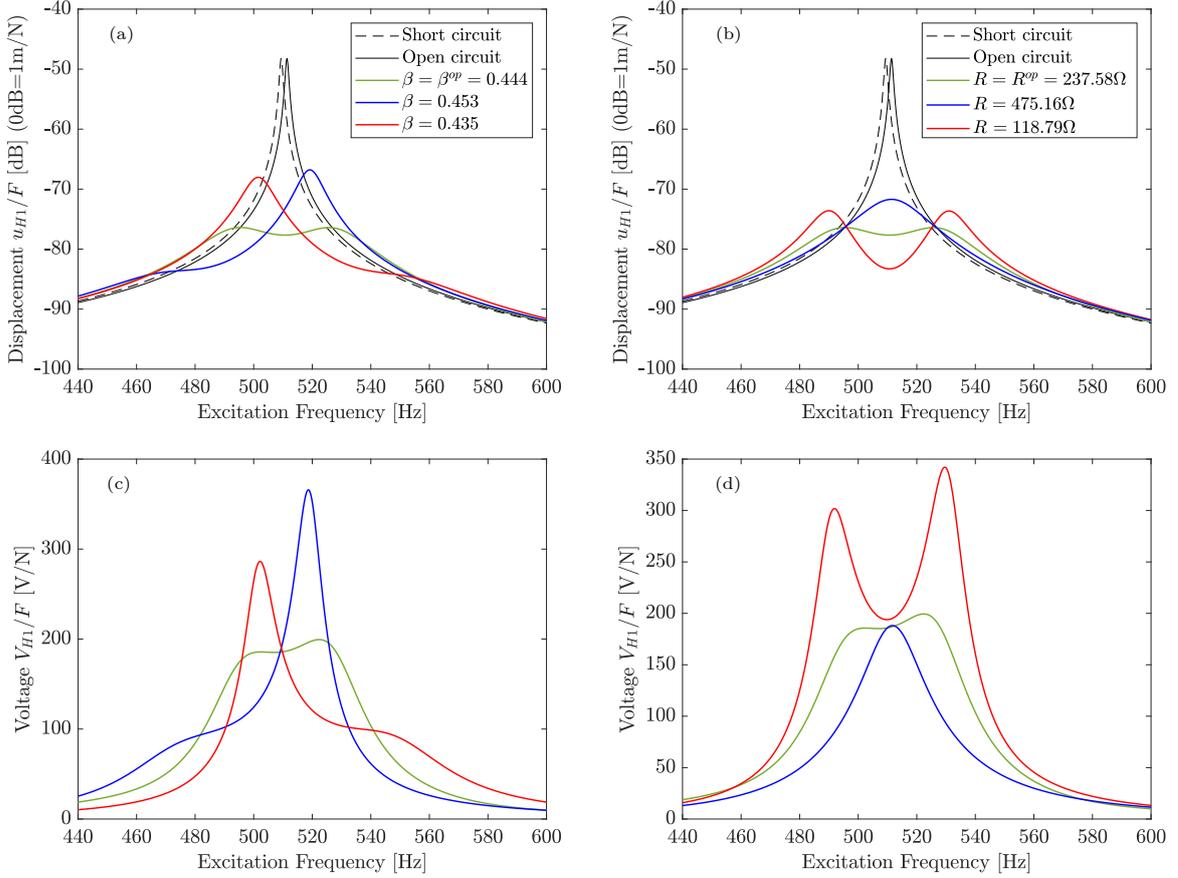
Fig. 11: Numerical frequency response of the first harmonics of  $u_{H1}$  (a,b) and  $V_{H1}$  (c,d) of  $u(t)$  and  $V(t)$ , both normalized by the excitation level  $F$ . The response is shown for different values of  $\beta$  with  $R = R^{op} = 237.58\Omega$  (a,c) and different values of  $R$  with  $\beta = \beta^{op} = 0.444$  (b,d). The modal parameters used are the ones gathered in Table. 3 and  $L = 0.737H \Leftrightarrow r = \omega_e/\hat{\omega} = 2$ .
