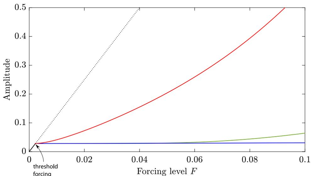
**Fig. 10** Fundamental harmonic amplitude  $X_{21}$  of  $X_2(t)$  as a function of the excitation level  $F$ , computed numerically with a continuation method, in the perfectly tuned case  $\sigma = 0$  (i.e.  $\omega_2 = 2\omega_1$ ), and for an external excitation frequency  $\Omega = \omega_2$ , corresponding to the cases of Fig. 9. Black line: linear response with all nonlinear terms cancelled; blue line: only
