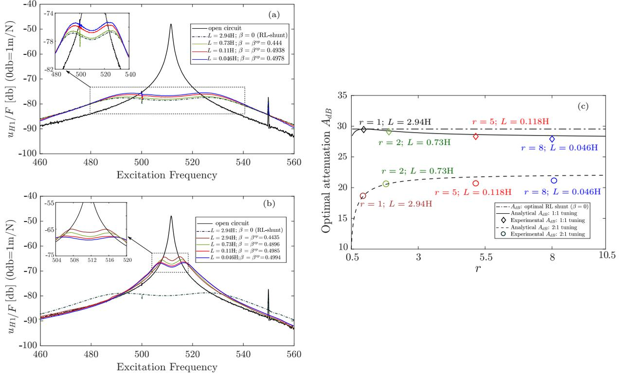
Fig. 23: (a) and (b) show the experimental frequency response of the first harmonic of the velocity  $u_{H1}$  for different values of the inductance for the 1:1 and 2:1 tuning, respectively. (c) Comparison between the optimal analytical attenuation and that measured experimentally for both tuning cases.
