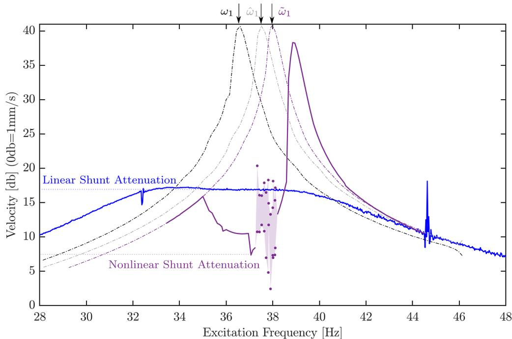
**Figure 16.** Comparison between the performance of the optimized linear shunt and the designed absorber for  $F = 2.5$  mN,  $\beta = 0.035$ , and  $\xi_1 = 0.0055$ . The dashed curves depict the linear responses for the short circuit case (black), the open circuit case (brown) and  $\beta = 0$  (purple). The solid lines depict the responses for  $\beta = 0.035$  (purple) and for the optimized linear shunt (blue).
