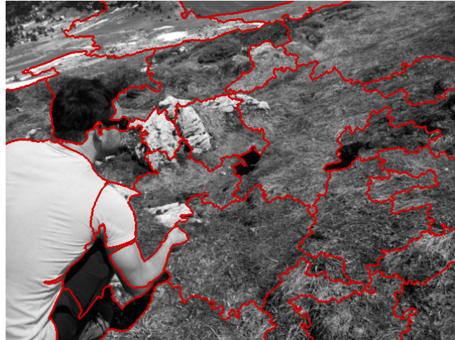
(a) Watershed segmentation using the gradient of T_{1000}^{a,\alpha}(f - 127.5)
