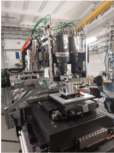
(a) Tensile testing machine and X-ray detector
