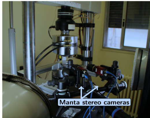
Figure 5.3: Experimental setups and measure devices for quasi-static tensile tests. (from [Davaze, 2019])
