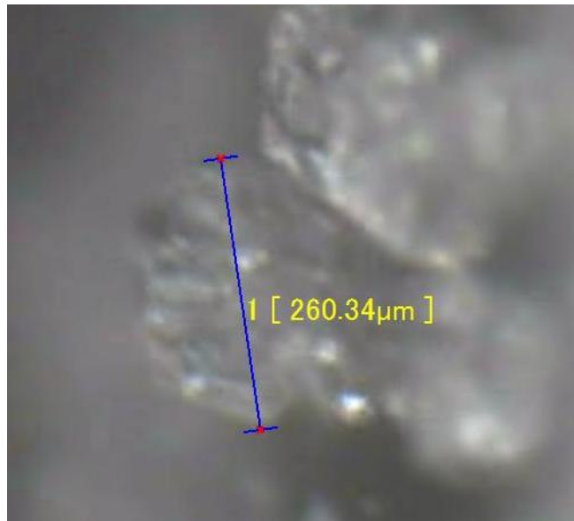
Figure 3.41: Solid CO 2 spherical crystal (magnification: 200X).
