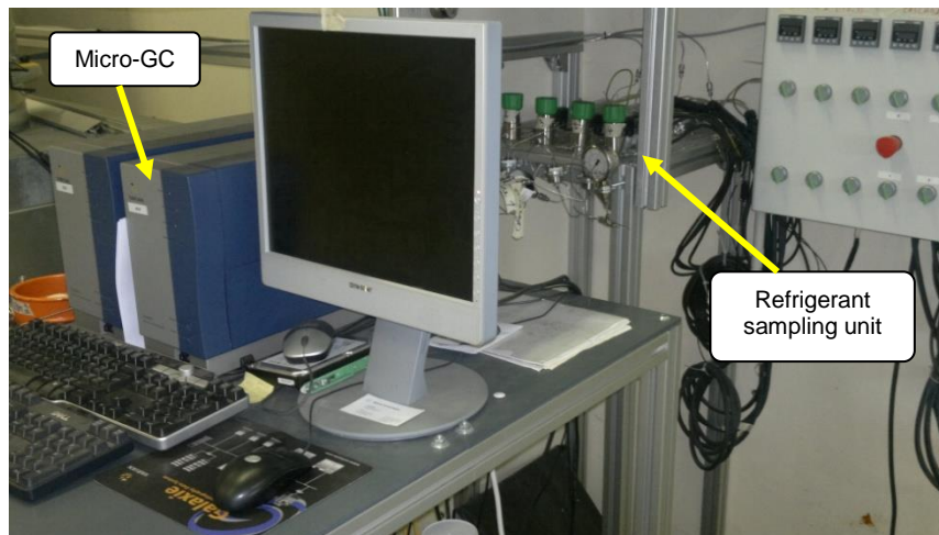
Figure 3.21: CP-4900 Micro-GC and sampling system.
