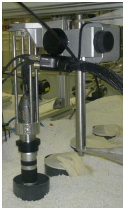
Figure 3.27: Step-by-step motor, camera and objective.
