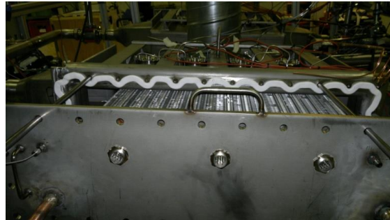
Figure 3.8: CFX installation in the enclosure.
