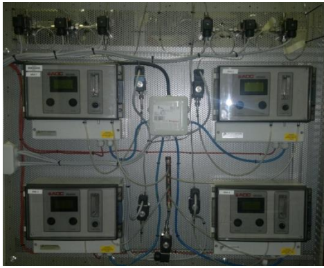
Figure 3.19: ADC SB 2000 gas analyzers. Figure 3.20: Flue-gas sampling from the CFX enclosures.
