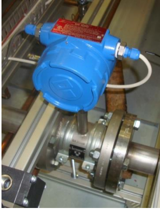
Figure 3.17: Thermal flue-gas mass flowmeter.
