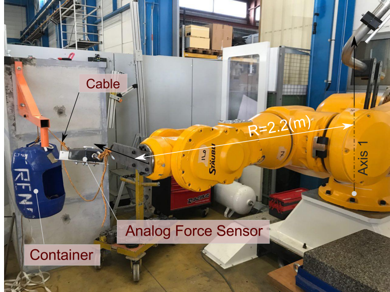
FIGURE 3.8: Force imposition method for stiffness identification of joint 1
