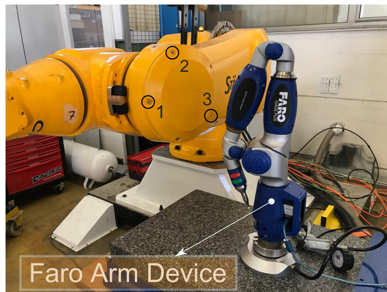
FIGURE 3.7: Illustration of measurement details of axis 1 stiffness identification using Faro arm
