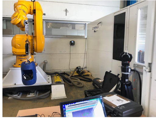
FIGURE 3.22: Measurement Setup for Elastostatic Model verification
