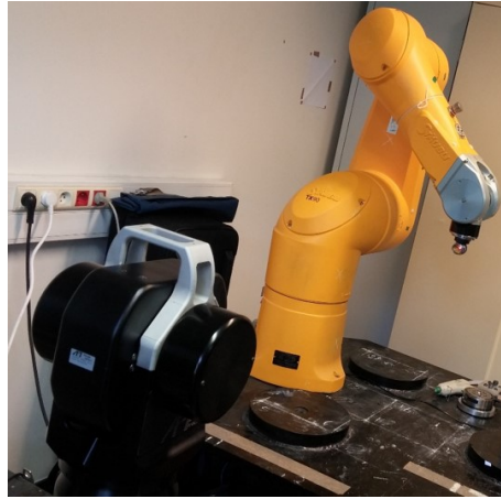
FIGURE 3.32: Experimental setup and Measurement device for identification of gear transmission errors executed in LISPEN laboratory
