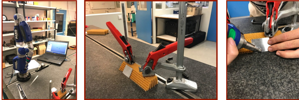
FIGURE 4.17: Installation of the Workpiece for measuring the chamfering angle in Steady State zone
