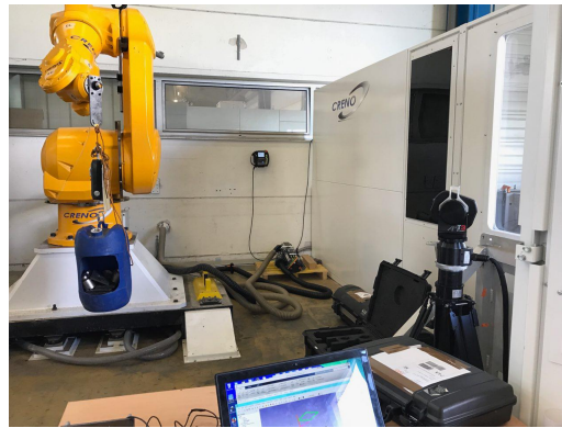
FIGURE 3.22: Measurement Setup for Elastostatic Model verification
