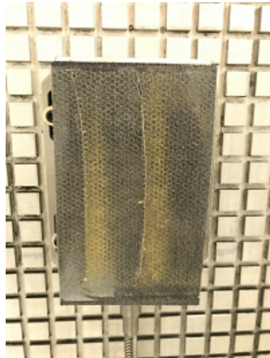
FIGURE 4.11: Penetration of knife in the protective moquette
