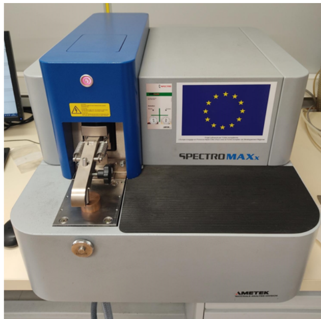
Figure 2.8 – Ametek SpectroMAXx® BT MX5M spark optical spectroscopy (spark-OES).
