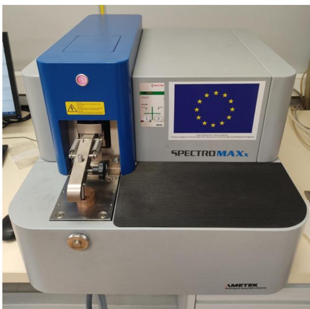
Figure 2.8 – Ametek SpectroMAXx® BT MX5M spark optical spectrometer (spark-OES).
