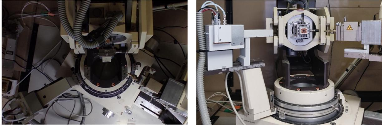
Figure 2.5 – Seifert XRD3000 used for X-ray diffraction.
