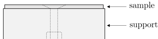
Figure 2.9 – Assembly of thin samples for spark spectrometer analysis.
