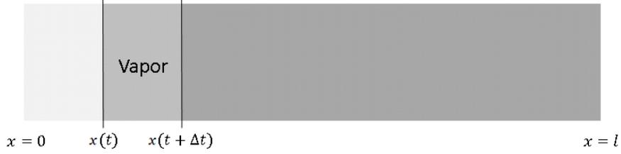
Figure 4.2: Volume that has vaporized between  $t$  and  $t + \Delta t$
