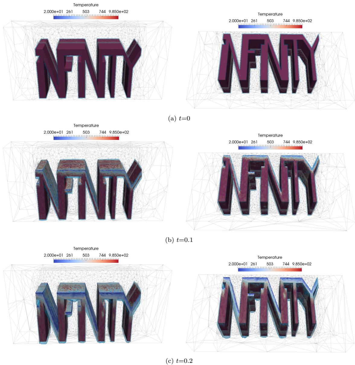
Figure 4.15: Evolution of the temperature at the solid interface and the dynamics of the interface separating water and vapor with a view from above (left) and below (right) at different time of the quenching of a complex geometrical solid
