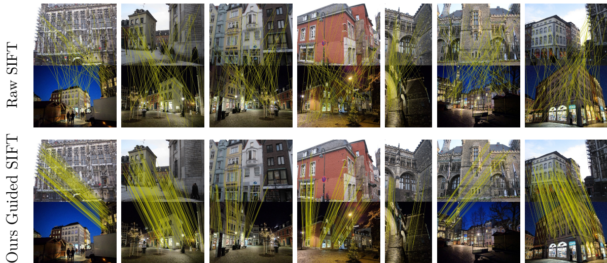
Fig. 3.4 Example of matching for SIFT with and without our method on Aachen daynight Sattler et al. (2018) . Learned guided matching is able to correctly match keypoints in difficult conditions when the descriptor alone is not.
