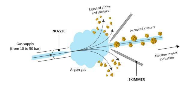
Figure 2.18. Schematic diagram of the formation of aggregates by adiabatic expansion of a gas. [174]
