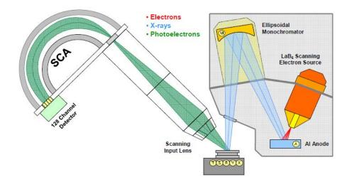
Figure 2.35. Schematic view of a monochromatized XPS instrument with a hemispherical energy analyser (HSA) and multi-channel detector.
