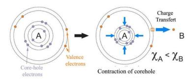
Figure 2.31. Schematic representation of the binding energy on a core-level before photoemission effects. When the A atom loses a valence electron for a more electronegative B atom, the binding energy of core-level electrons in the A atom increases.
