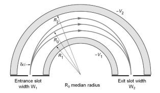
Figure 2.38. Scheme of a 180° hemispherical analyser commonly used in XPS. [184]
