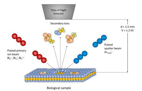
Figure 2.11. ToF-SIMS principle showing a bismuth primary ion beam colliding with the surface of a biological sample and generating characteristic secondary ions. The incidence of an argon cluster sputter beam with the surface of the sample is also illustrated.
