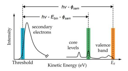
Figure 2.41. Schematic of a full photoemission spectrum. The intensity of the collected photoelectrons is plotted as a function of kinetic energy. The coloured areas represent the high intensity photoemission threshold corresponding to secondary electrons of low kinetic energy (blue), the core level region (green) and the valence band (orange). Adapted from [191]
