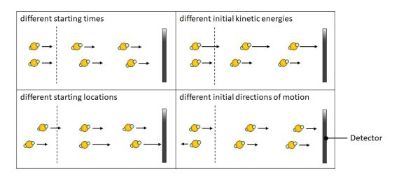
Figure 2.21. Factors affecting mass resolution in a linear ToF mass analyser. [174]
