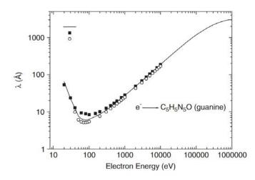
Figure 2.29. Inelastic mean free path  $\lambda(E)$  results for incident electron energies in guanine. –, experimental study; and  $\circ$ , theoretical results. [183]
