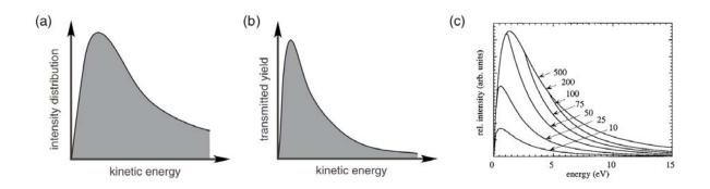
Figure 2.44. Schematic secondary electron spectrum before (a) and after passing through the electron emission microscope optics (b). (c) Energy distribution of electrons transmitted through a PEEM column using apertures of different diameters (in  $\mu$ m). [193, 194]
