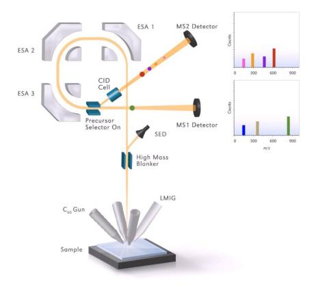
Figure 2.23. Schematic of the PHI nanoTOF II with MS/MS. [177]
