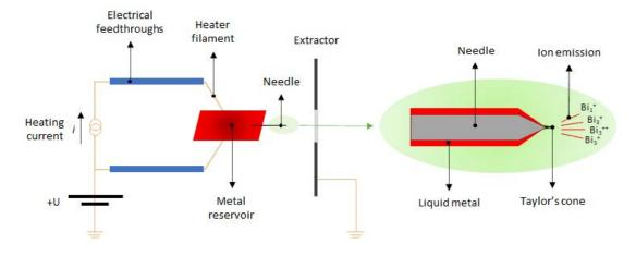
Figure 2.15. Schematic view of a LMIS emitter. [172]
