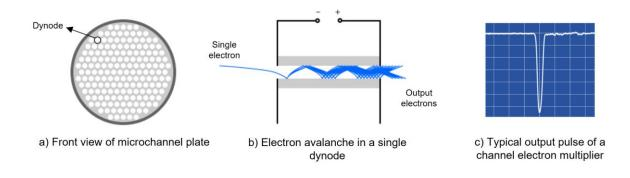
Figure 2.40. Front view of a microchannel plate, the generation of an electron avalanche with a single incident electron, and the typical output pulse of a channel electron multiplier.
