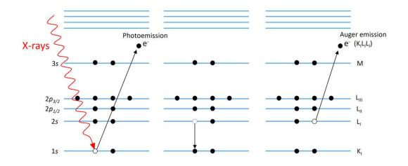
Figure 2.33. Auger transition principle for a KLL emission. [189]
