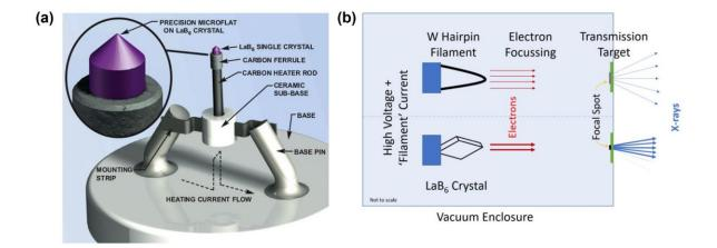
Figure 2.36. (a) Schematic view of a Lanthanum Hexaboride (LaB<sub>6</sub>) cathode used in an X-ray source for XPS equipment. (b) Schematic of a comparison of open, transmissive-target X-ray tubes using either a traditional Tungsten (W) hairpin filament or LaB<sub>6</sub> crystal for electron generation and the relative effects these have on focal spot size and X-ray emission (flux). Emission is actually from almost 180° from the target exit surface but ray diagram is simplified for clarity.
