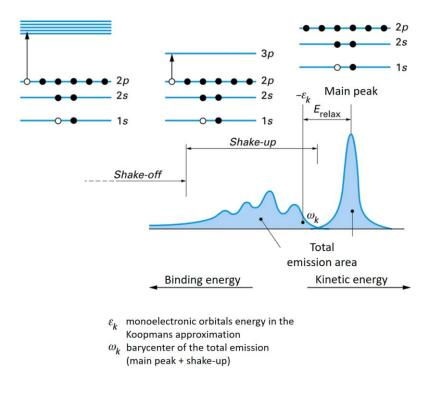
Figure 2.34. Shake-up and shake-off process. [184]
