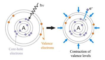
Figure 2.32. Schematic representation of the binding energy on a core-level after photoemission effects. When a core-hole is created in an A atom due to a photoemission process, the valence levels contract to compensate the positive charge and, consequently, the binding energy of core-level electrons in the A atom decreases.
