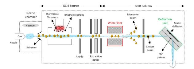
Figure 2.17. Schematic configuration of GCIB. [173]
