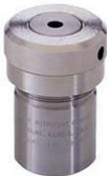
Figure 1 : Photograph of a Parr company reactor used for hydrothermal synthesis.
