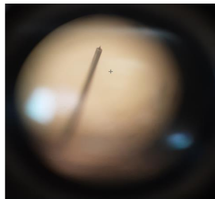
Figure 2.13: (a) assembly for electrochemically cutting the tip, (b) final shape of a tip STM
