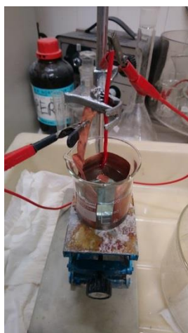
Figure 2.10: Electrochemical polishing cell of copper
