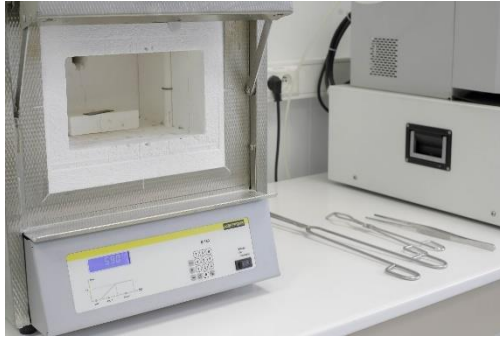
figure B-2: Four à moufle Nabertherm L 5/11/B180
