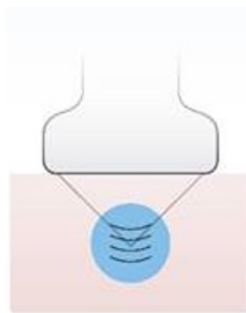
FIGURE 2.9: Acoustic radiation force principle: ultrasound probe sends focused ultrasounds to create shear waves that propagate transversely to the ultrasounds sent (from Sigrist et al., 2017).
