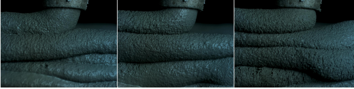
Figure 4.8: Examples from the I3DCP dataset: the first, middle and last image, respectively from left to right. The dataset is ordered chronologically.
