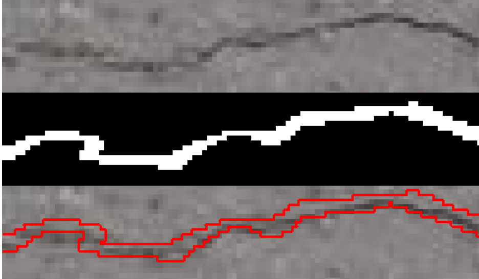
Figure 3.1: A zoom to errors on the level of pixels in the CrackForest dataset. The first row shows the raw image, the second one shows a manual annotation, and the third one shows the image with a red border surrounding the annotation.
