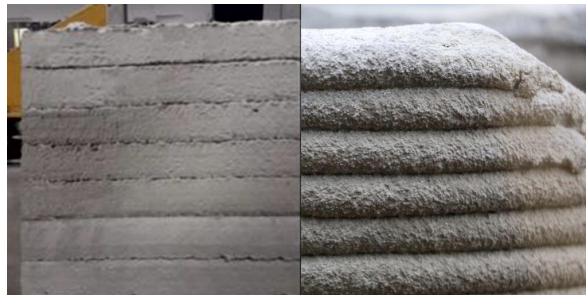
Figure 4.9: Comparison of wide rectangular extrusion (left) as illustrated by (Davtalab et al. [2020]) and thin cylindrical extrusion (right) as used in our experiments.
