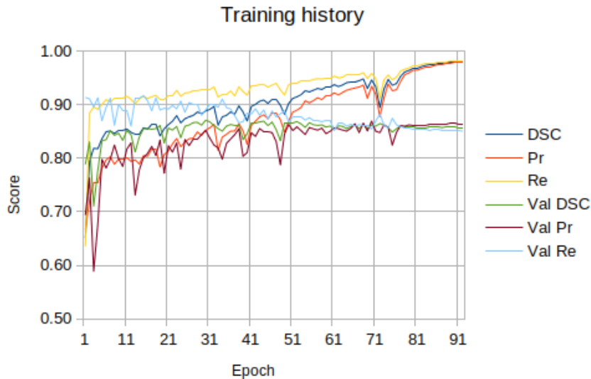
Figure 4.13: Evolution of the evaluation scores in the training and the validation sets, during the training of m_1 using manual annotations ( T_S ).
