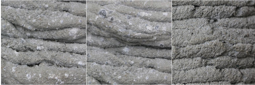
Figure 4.2: Examples of bad quality pieces in which the interlayer lines are difficult to recognize.
