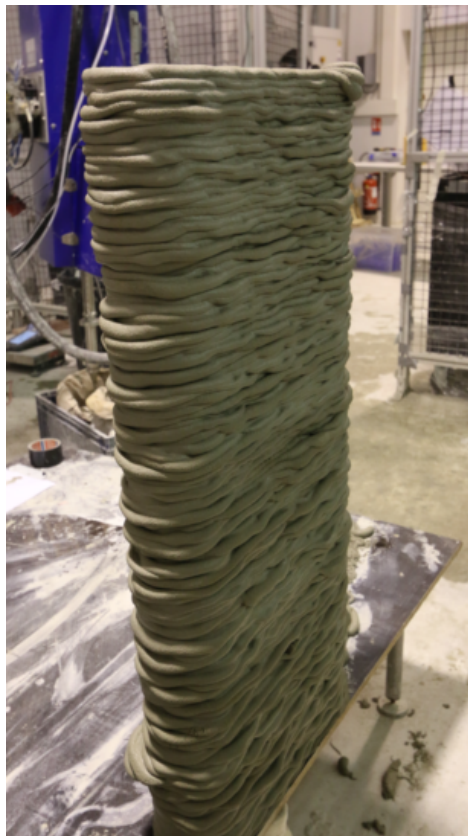
Figure 4.5: The experimental sample printed with purposely created defects.
