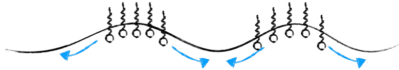
Fig. 1.16 Gibbs elasticity: stabilisation of the capillary waves because of enhanced elasticity in the presence of insoluble surfactant monolayers
