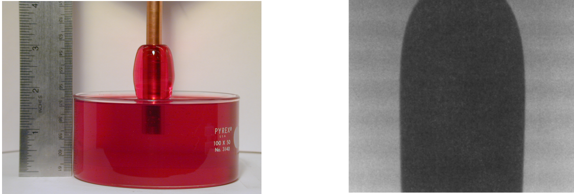
Fig. 1.12 a) A dilute (0.025 wt%) solution of a high molecular weight (2106 g/mol) polystyrene polymer (Polysciences Inc) is dissolved in a low molecular weight (100 g/mol) newtonian viscous (30 Pa.s) solvent (Piccolastic, Hercules Inc). The polymer solution climbs a rod when the rod is rotated inside the solution, as can be seen in the image, an effect called the Weissenberg effect (courtesy of J. Bico and G. McKinley, MIT). b) Die-Swelling is the effect of increasing jet diameter as it comes out of the orifice because of the presence of polymeric particles in the solution (courtesy of C. Allain, M. Cloitre, P. Perrot, FAST [27]).
