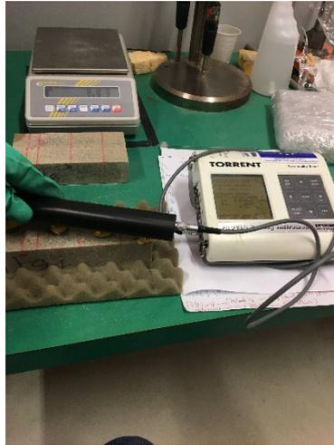
**Figure 57.** Mesures non-destructives : Méthode ‘The Wenner resistivimeter’.
