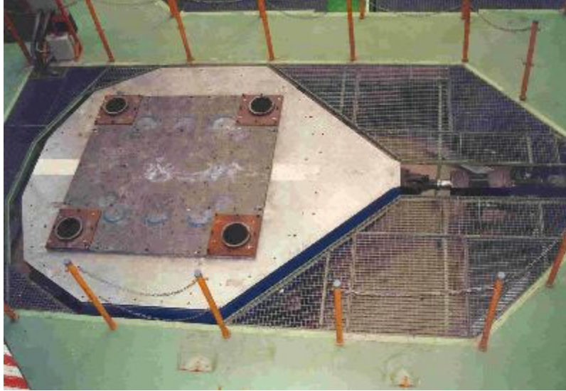
Figure 5.17 General view of Vésuve shaking table at CEA ( Vesuve.jpg (400×274) (cea.fr) ).
