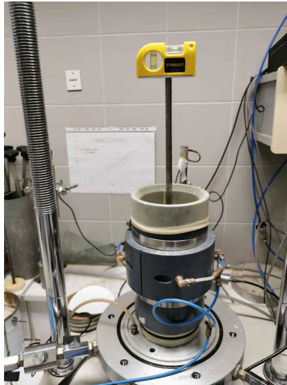
Figure 2.6 View of the membrane-lined split mould during specimen reconstitution process.
