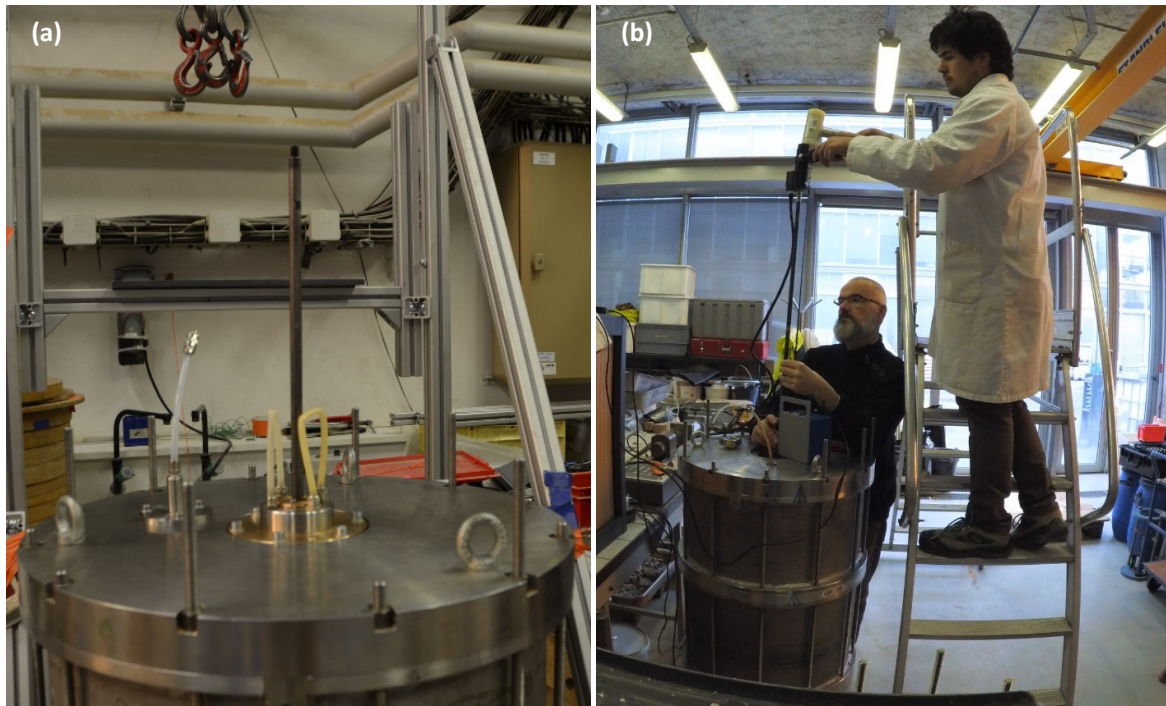
Figure 2-35 – Dynamic penetration test: (a) penetrometer rod train installation; (b) penetrometer installed and dynamic driving.
