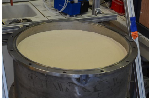
Figure 2-31 – Reconstituted sand specimen.
