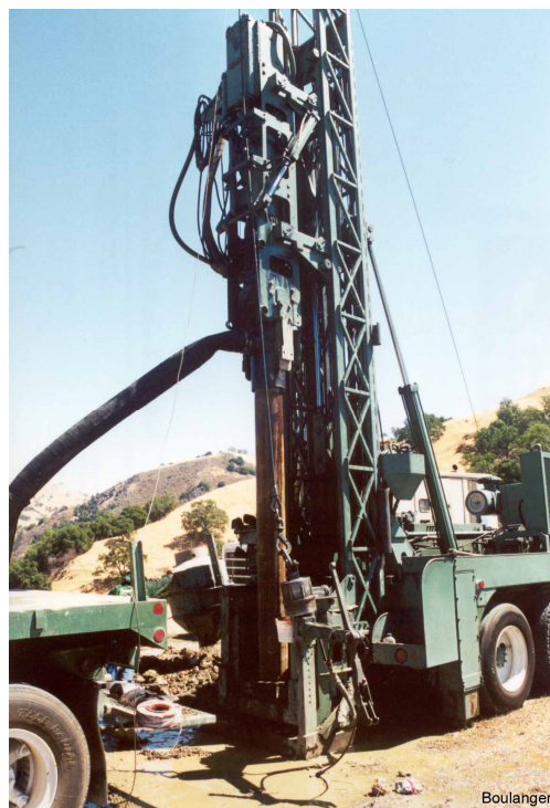
Figure 1-35 - Becker penetrometer (UCD 2022).
