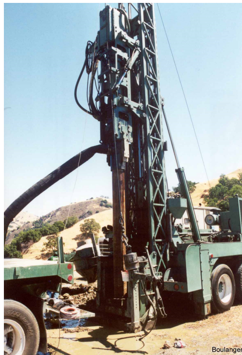
Figure 1-35 - Becker penetrometer (UCD 2022).
