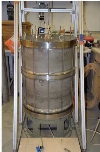
Figure 2-24 – View of the K_0 calibration chamber of Navier laboratory.
