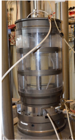
Figure 4-5 – Adjustment of the lateral confinement chamber.
