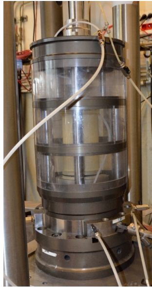
Figure 4-5 – Adjustment of the lateral confinement chamber.
