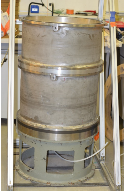
Figure 2-26 – Cylindrical mold of K_0 calibration chamber.
