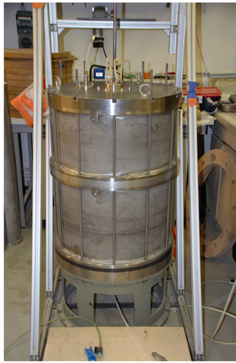
Figure 2-24 – View of the K_0 calibration chamber of Navier laboratory.
