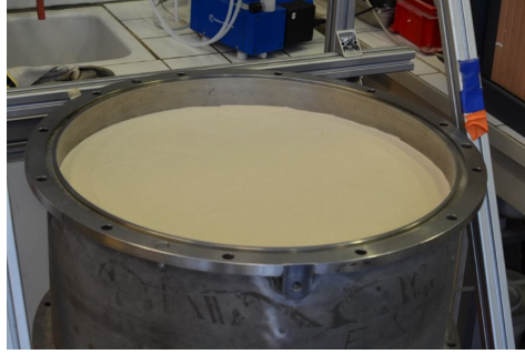
Figure 2-31 – Reconstituted sand specimen.
