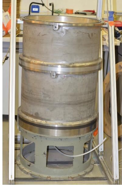
Figure 2-26 – Cylindrical mold of K_0 calibration chamber.
