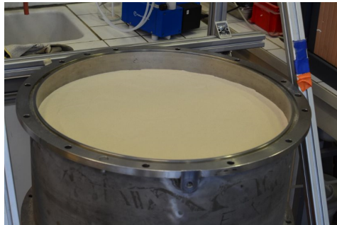
Figure 2-31 – Reconstituted sand specimen.
