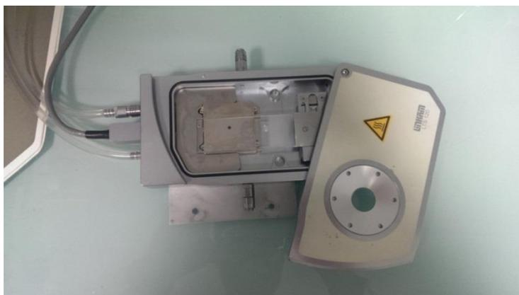
Figure 38. Photo de la platine chauffante LTS120.
