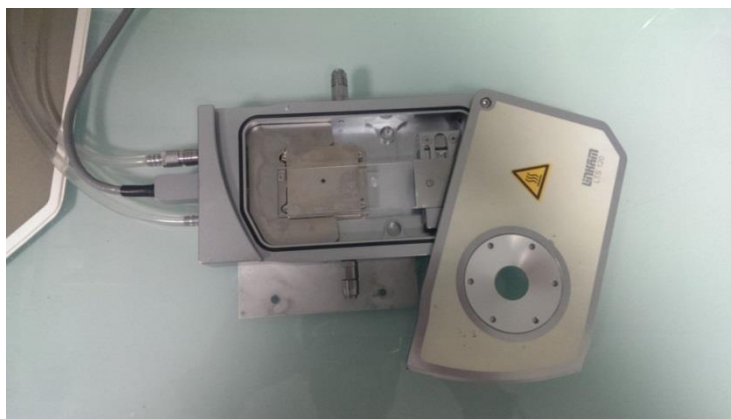
Figure 38. Photo de la platine chauffante LTS120.
