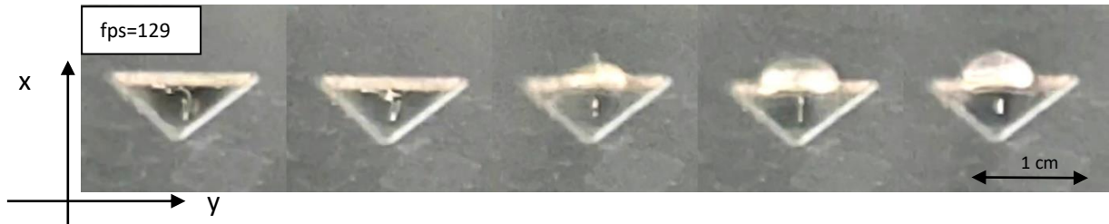
Figure 4.8: Time evolution of the fundamental resonant mode within a triangle perforation, f=87 Hz and \Delta t = 1/129 s.
