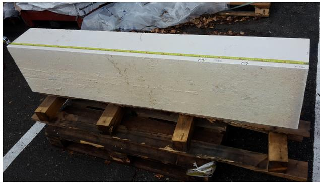
Figure 1.1: Photo of a new block (1600 x 400 x 250 mm).
