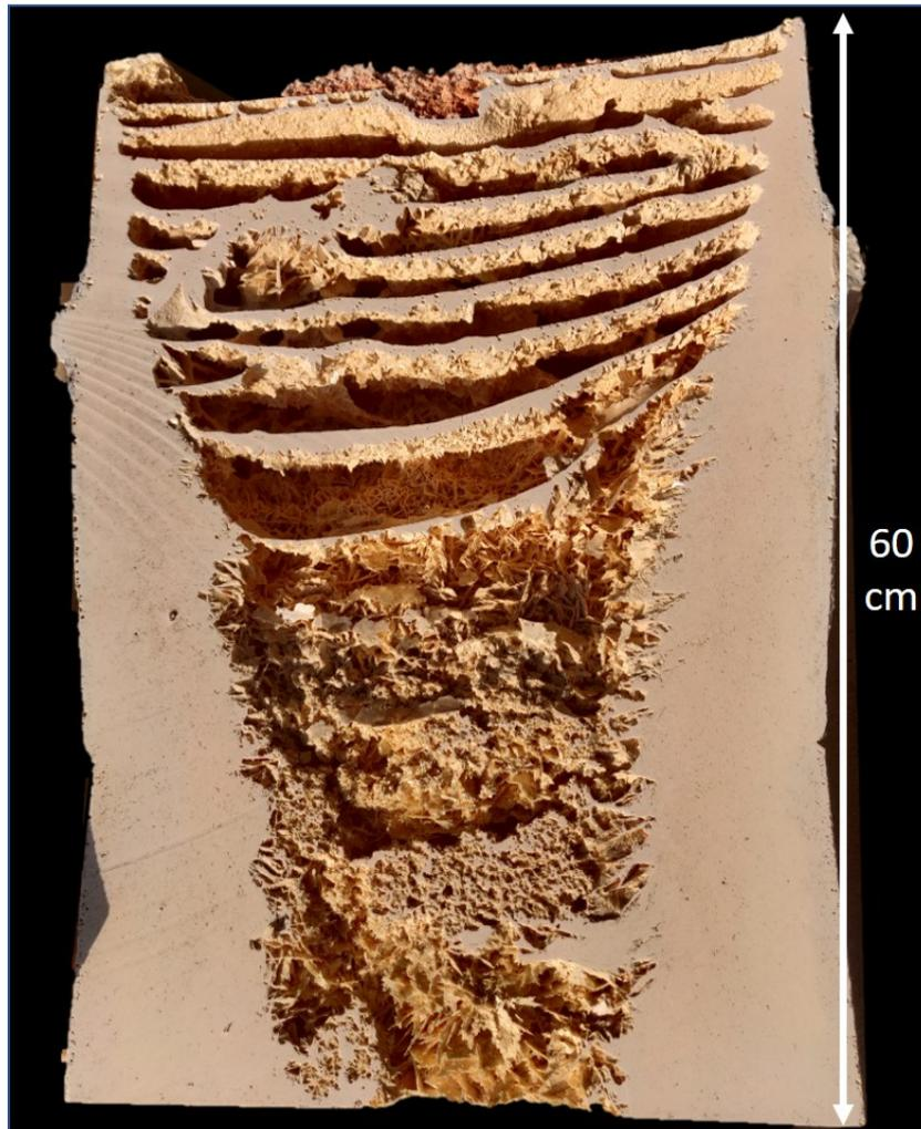
Figure 3.21: Macro-porosity inside an industrial riser of an AZS block with 41 wt.% of  $ZrO_2$ .
