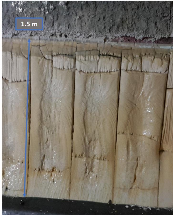
Figure 1.4: Blocks installed in a furnace at the end of its life.
