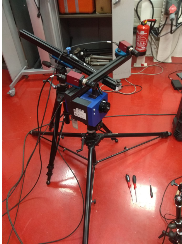
FIGURE 2.6: Two stereo correlation cameras (red) on top of the infrared camera (blue).
