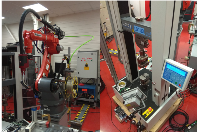
FIGURE 2.4: Machines needed for a PVR experiments. On the left, TIG welding torch attached to a robotic arm. On the right, tensile loading machine.
