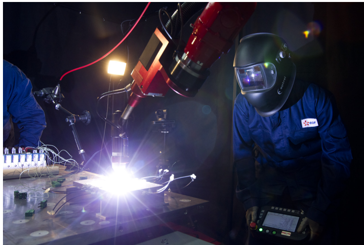
FIGURE 1.1: Automatised Tungsten Inert Gas (TIG) welding experiment at EDF R&D's welding lab.
