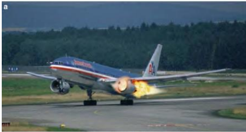
Figure 1-3: compressor surge leading to a flameout (source: El-Sayed A.F 2015)
