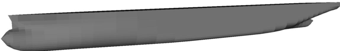
Figure 95 - Watertight volume of the 110-metre tanker
