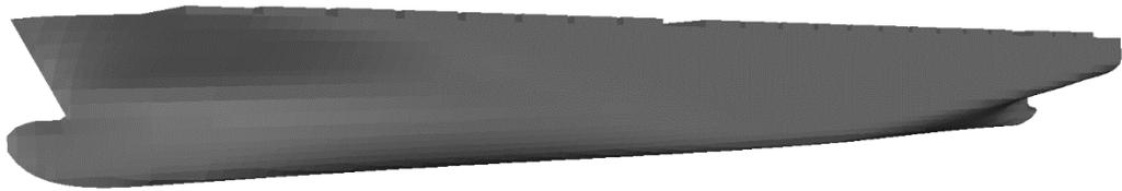
Figure 87 - Watertight volume of the 14400 TEU container ship
