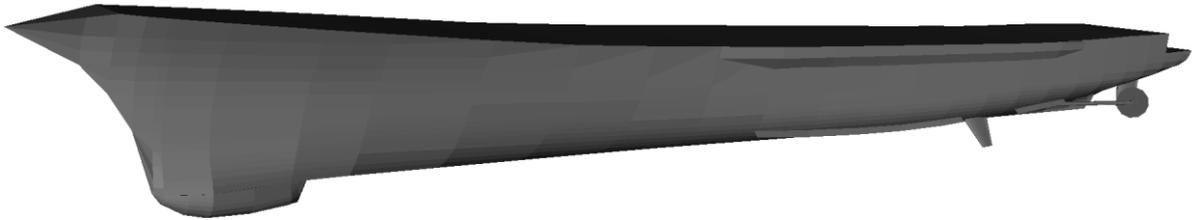
Figure 100 - Watertight volume of the FASM
