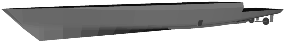
Figure 97 - Watertight volume of the OPV
