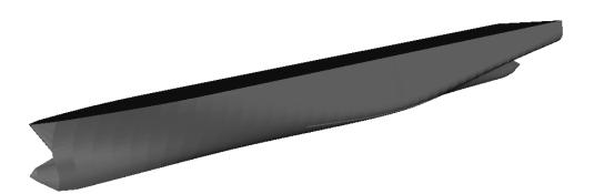
Figure 83 - Watertight volume of C11-class container ship (4832 TEU)
