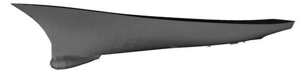
Figure 99 - Watertight volume of the open form DTMB-5415
