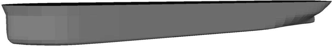
Figure 96 - Watertight volume of the 227.5-metre tanker
