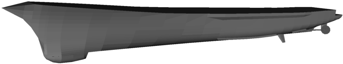
Figure 100 - Watertight volume of the FASM
